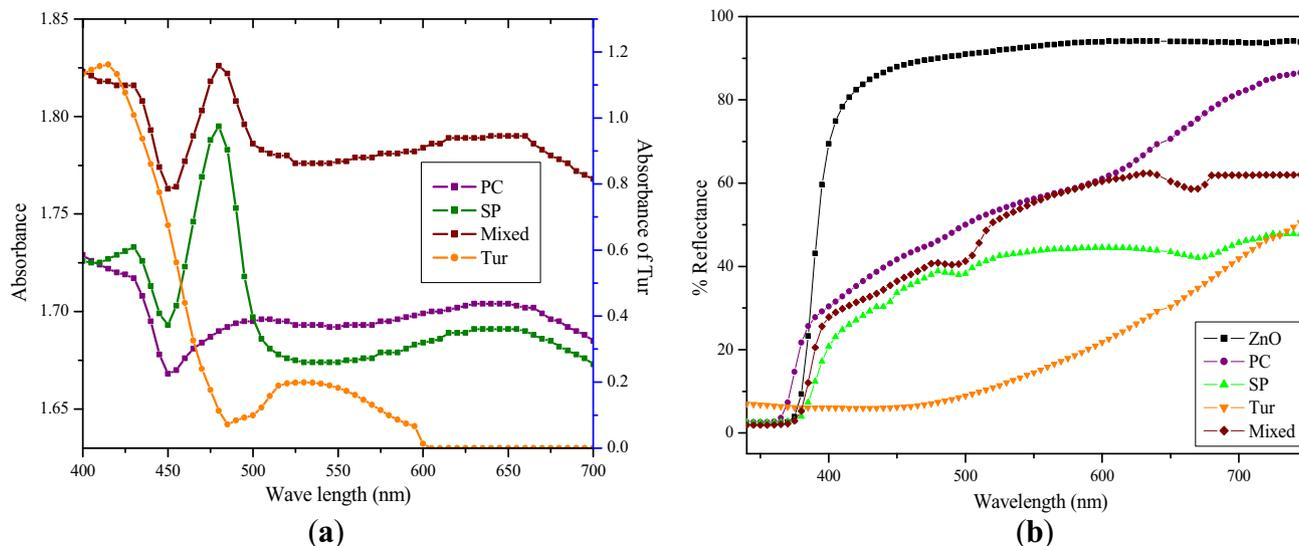
**Figure 5.** (a) UV-Vis absorption spectra of purple cabbage, spinach, turmeric and their mixed one with different peak positions; (b) DRS of Zinc oxide film with and without loading of different natural dyes show peak shifting.
