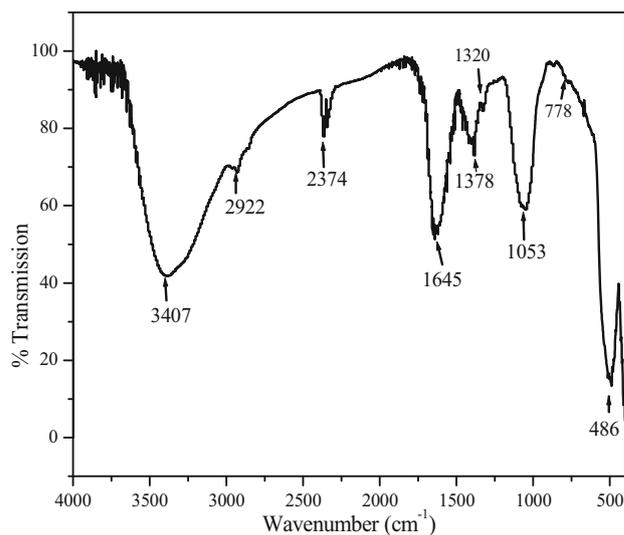
**Figure 4.** FTIR spectra of Mixed dye containing anchoring groups on ZnO substrate.
