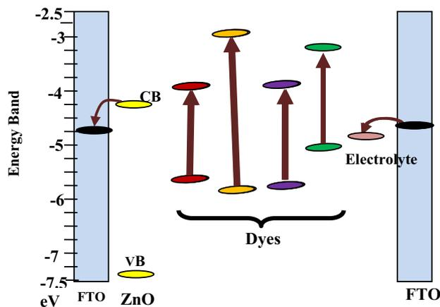
**Figure 9.** Energy band diagram of dye-sensitized solar cell with natural dyes and their mixture.
