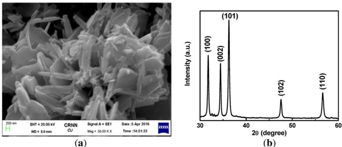
**Figure 3.** (a) FESEM image of the nanostructured ZnO coated on FTO glass; (b) XRD pattern of synthesized ZnO.
