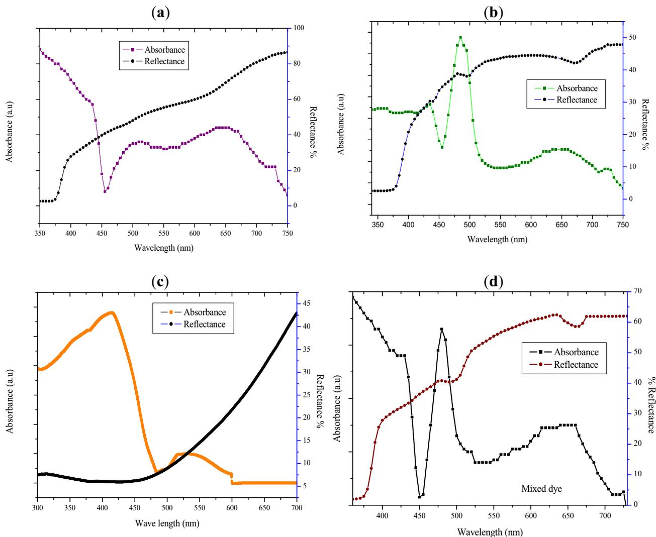
**Figure 6.** Comparison of UV-vis absorbance spectra of different dyes with their DRS, loaded with zinc oxide films. (a) Purple Cabbage (PC), (b) Spinach (SP), (c) Turmeric (Tur) and (d) Mixed of three dyes.
