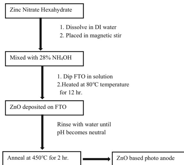
**Figure 1.** Flowchart for the synthesis of nanostructured ZnO photo anode.
