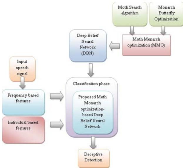
**Figure 1.** Block diagram of proposed MMO-DBN deception detection system.
