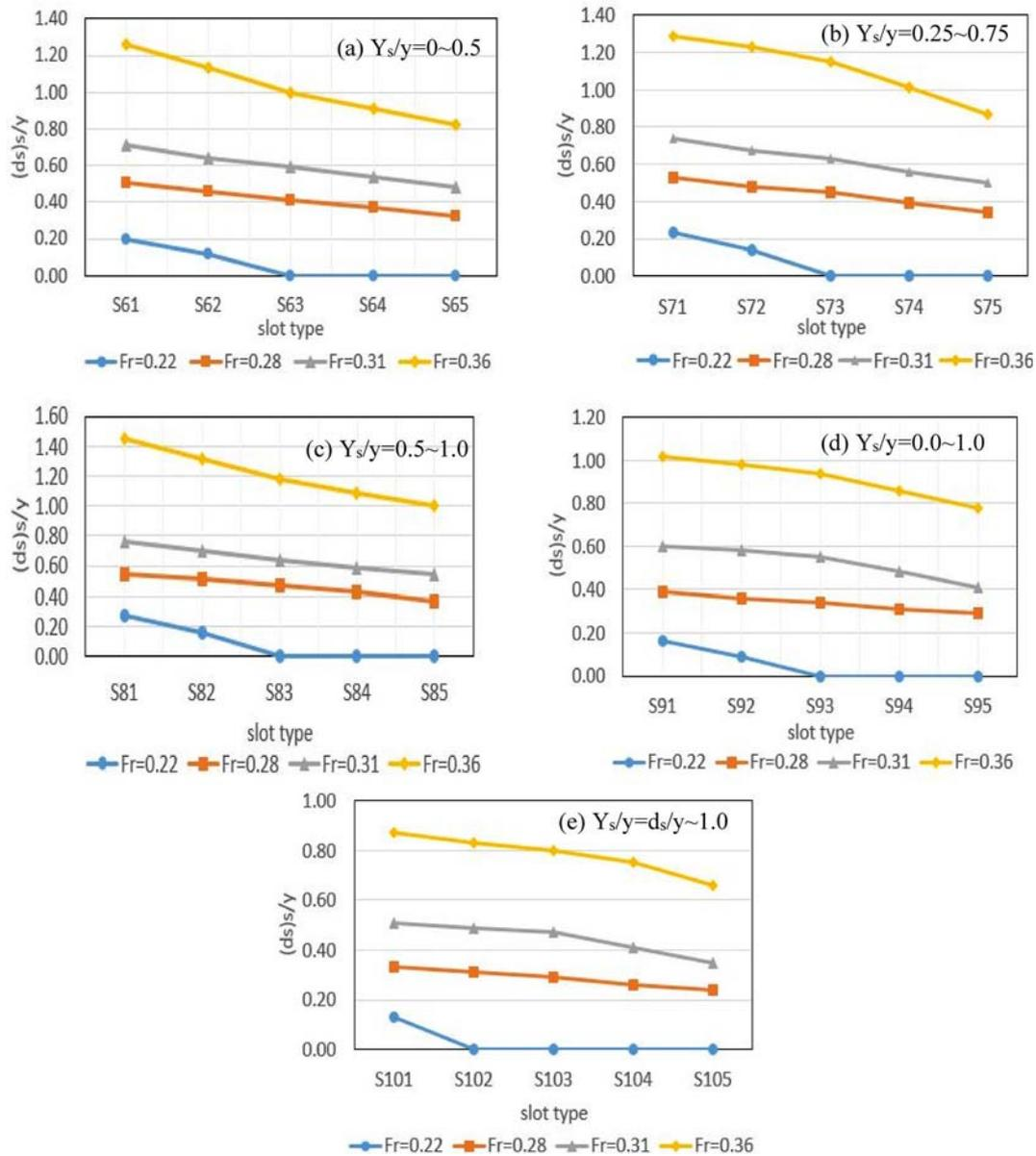
**Figure 7.** Dimensionless scour depth for different horizontal slot positions.
