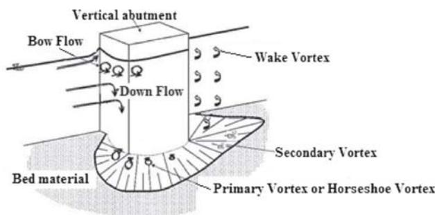
**Figure 1.** The flow field around a bridge abutment [7].
