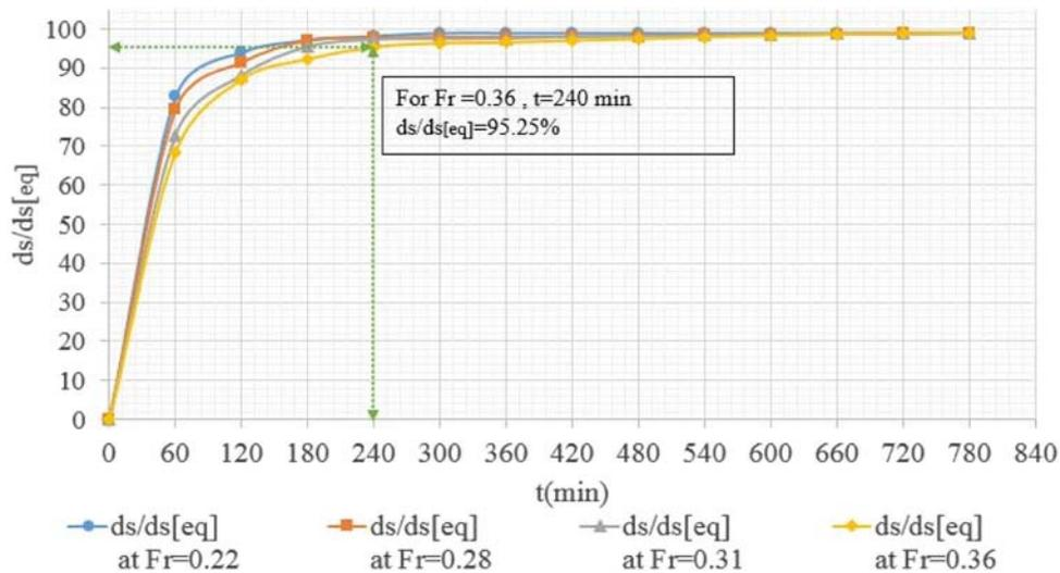
**Figure 4.** Equilibrium scouring time calculation curve for  $Fr = 0.36, 0.31, 0.28,$  and  $0.22$  in control experiments (scour depth to equilibrium scour depth ratio to time).
