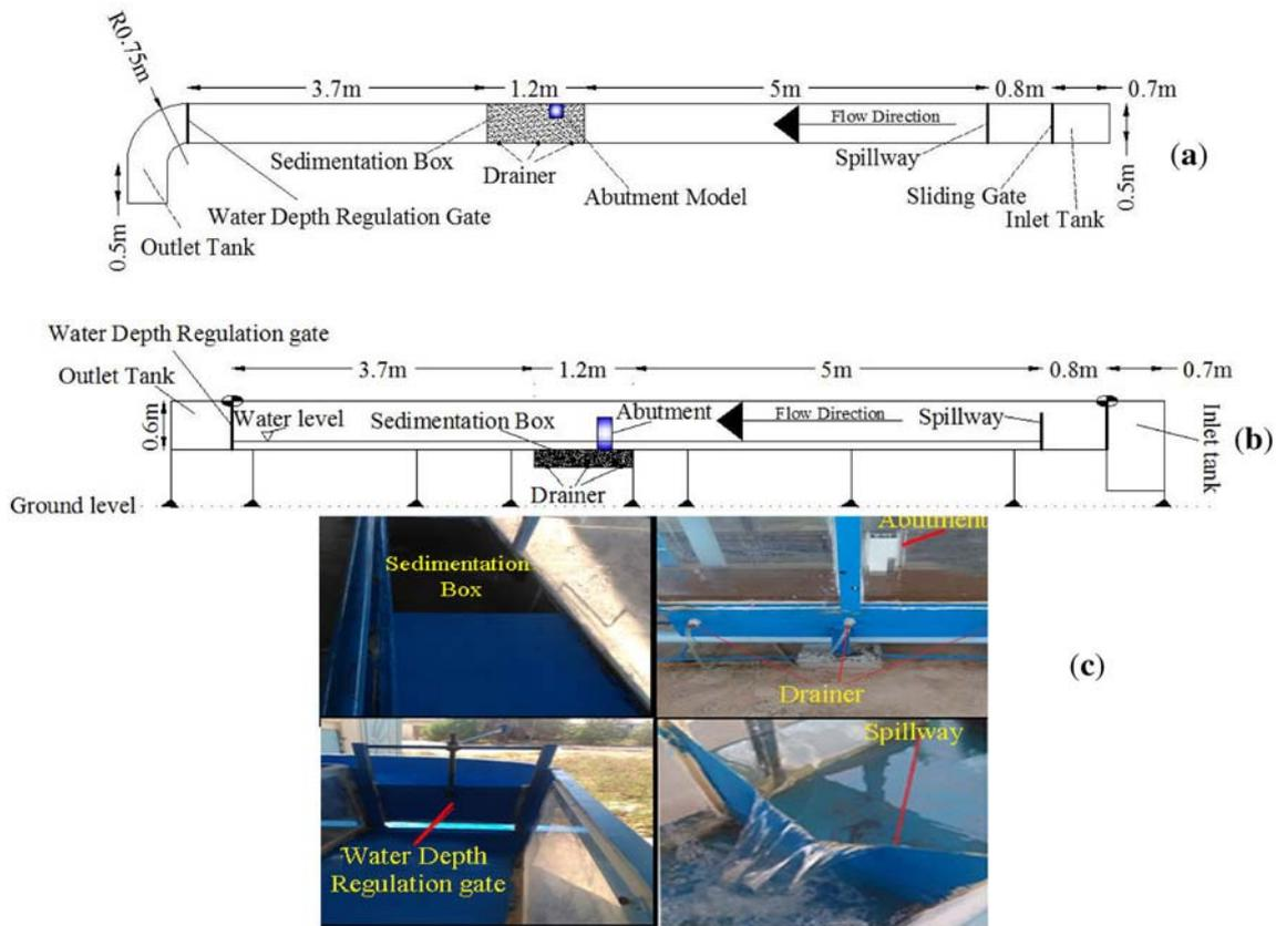
**Figure 2.** (a) Flume plan and experimental set-up, (b) cross-sectional view of the flume and (c) pictures of different parts of the flume.
