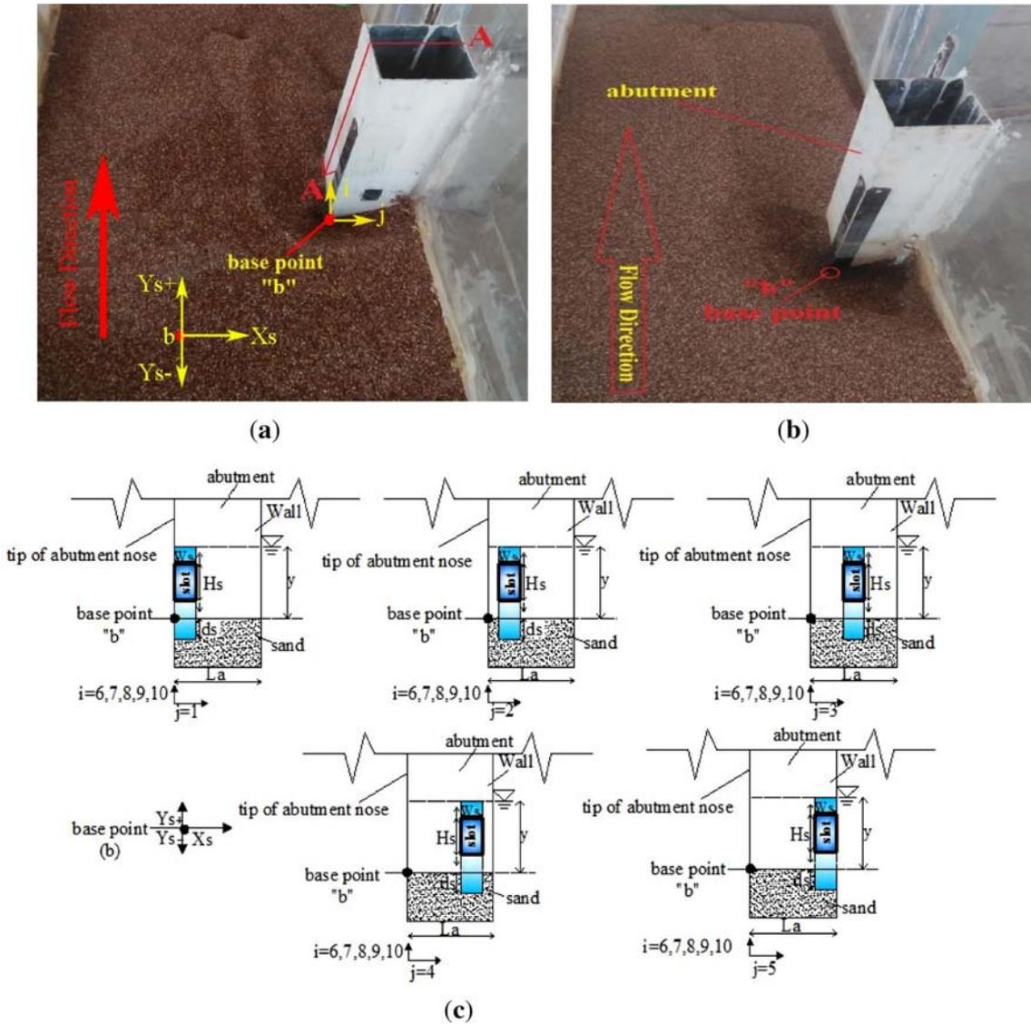
**Figure 3.** (a) An example of a model of abutment with a slot. (b) Display of base point (starting point of scour phenomenon and location of maximum scour depth). (c) Cross section A-A, different parameters of slot at different positions to the tip of abutment nose.
