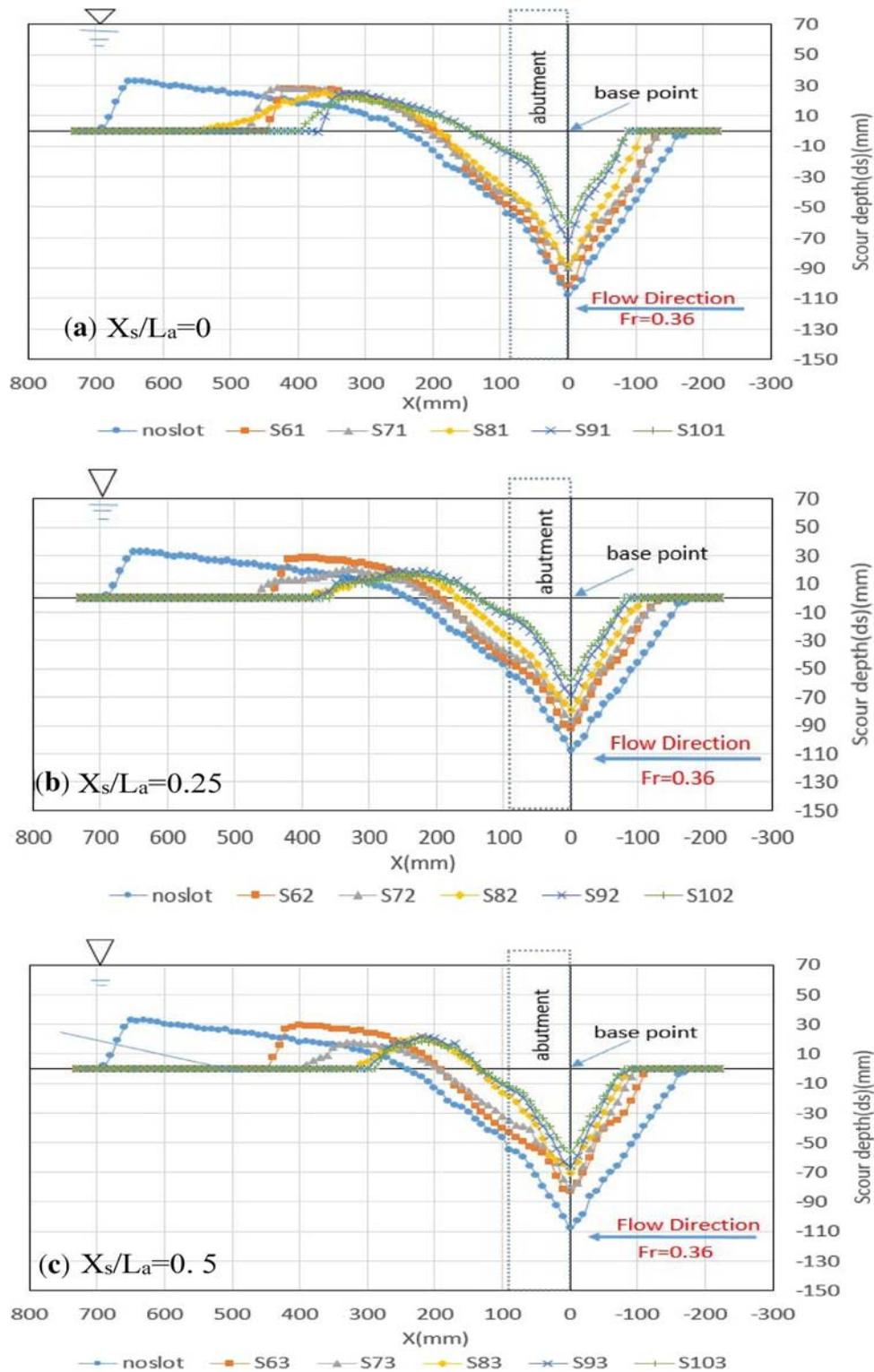
**Figure 5.** Comparison of the longitudinal profile of the scour around the abutment for  $Fr= 0.36$  and different vertical slot positions.
