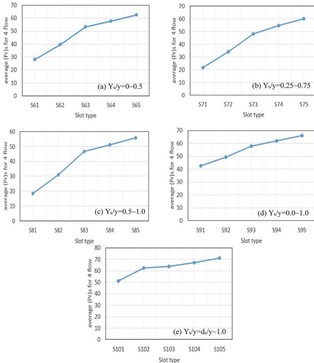
**Figure 8.** Average percentage of scour depth reduction for different horizontal slot positions.
