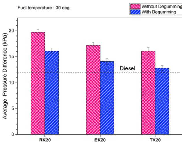
**Figure 5.** Pressure difference comparison at 30°C and 0.075 m<sup>3</sup>/h.
