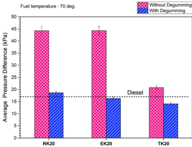
**Figure 7.** Pressure difference comparison at 70°C and 0.075 m<sup>3</sup>/h.
