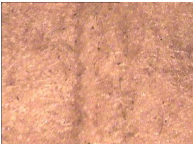
**Figure 11.** Surface morphology of the filter elements without the degumming process.
