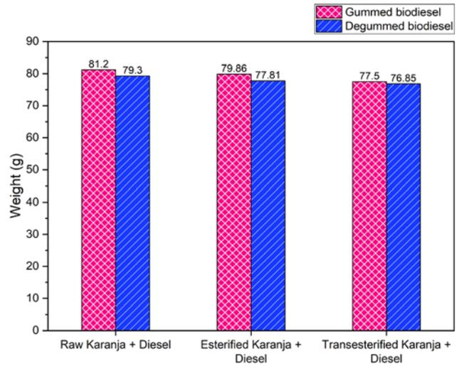
**Figure 9.** Effect of contaminants on the mass of fuel filter.
