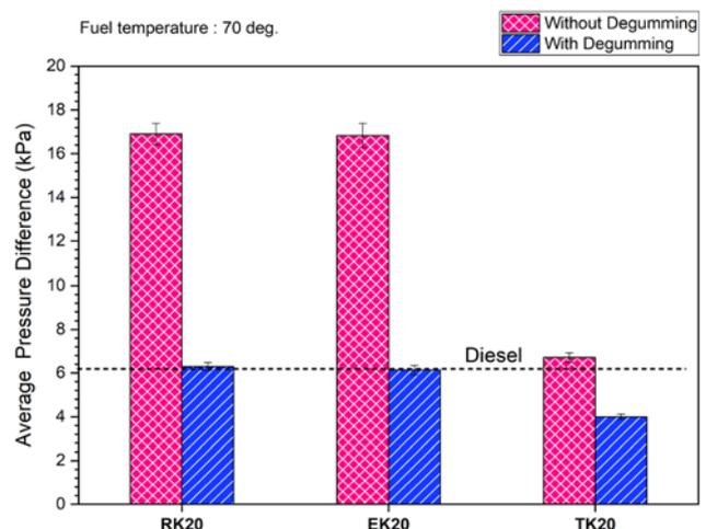
**Figure 6.** Pressure difference comparison at 70°C and 0.03 m<sup>3</sup>/h.
