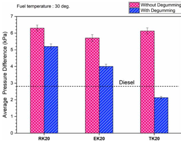
**Figure 4.** Pressure difference comparison at 30°C and 0.03 m<sup>3</sup>/h.
