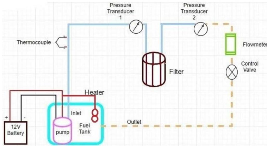
**Figure 1.** Schematic diagram of the experimental filter set-up.
