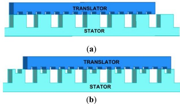
**Figure 5.** Basic structure (a) Stator with no notch, (b) Stator with notch.
