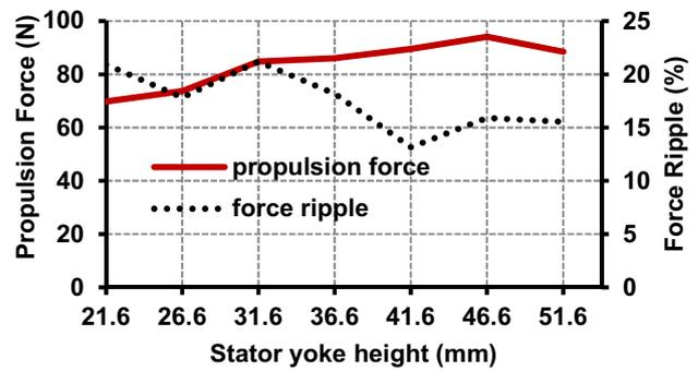
**Figure 11.** Performance variation with stator yoke height.
