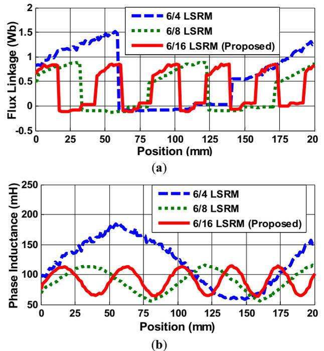
Figure 13. Comparison (a) Flux Linkage, (b) Inductance.
