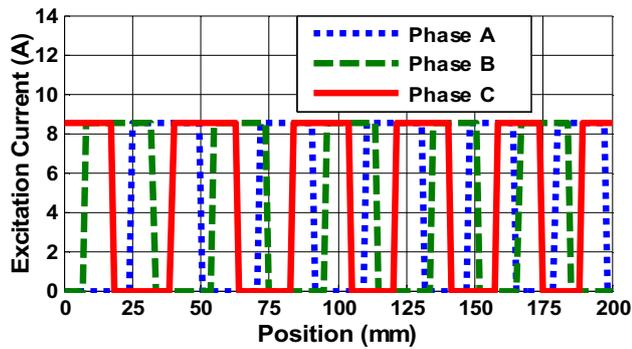
Figure 21. Three-phase excitation current for 6/16 LSRM.
