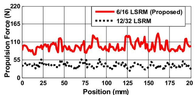
**Figure 20.** Propulsion force profiles of 6/16 and 12/32 LSRMs.
