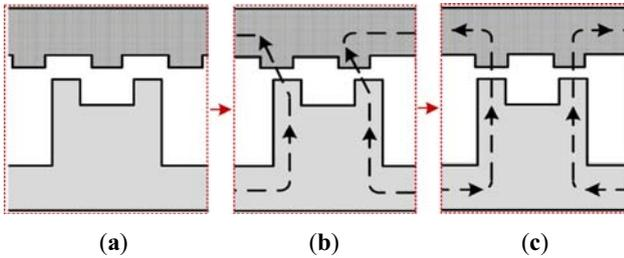
**Figure 2.** Operating principle LSRM (a) non-aligned position, (b) half-aligned position and (c) aligned position.
