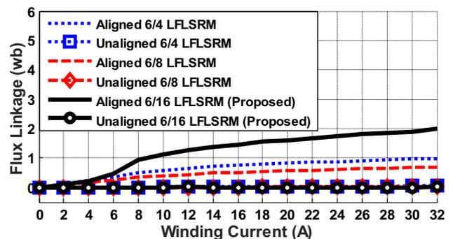
Figure 14. Flux current variation at aligned and non-aligned teeth position.
