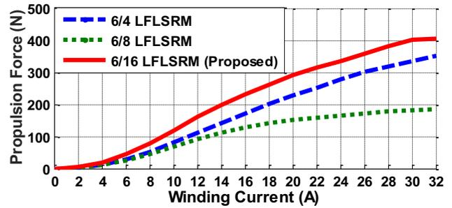
**Figure 16.** Force- current variation of the three motors.
