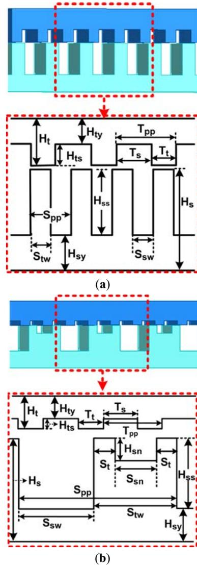
**Figure 4.** Design dimensions (a) Conventional LSRM, (b) Proposed LSRM.
