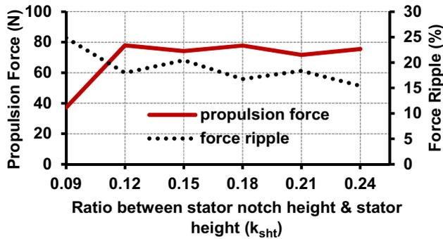
**Figure 7.** Performance variation with stator notch height.
