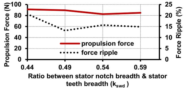
**Figure 9.** Performance variation with stator notch breadth.
