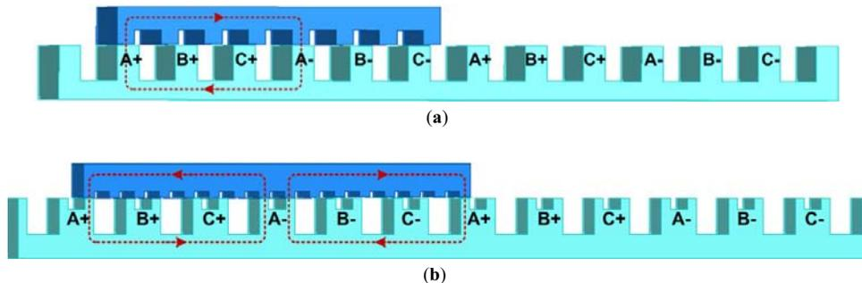
**Figure 3.** Flux path during aligned teeth position (a) Conventional LSRM. (b) Proposed LSRM.
