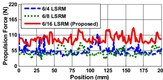
**Figure 17.** Propulsion force produced by the three motors.
