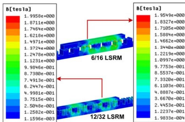
**Figure 18.** Flux density distribution at aligned teeth position.
