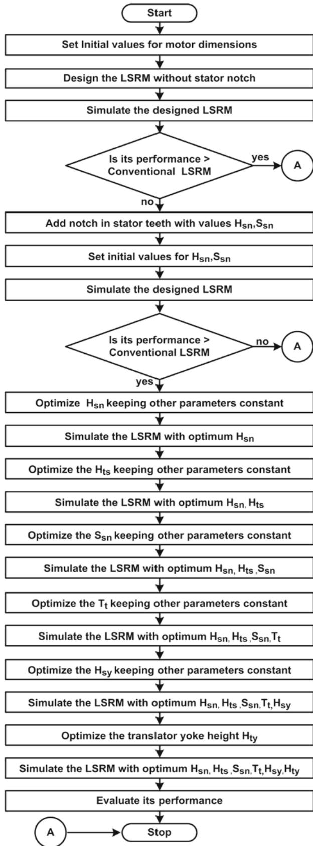
◀ **Figure 6.** Parameter based cumulative deterministic optimization algorithm.
