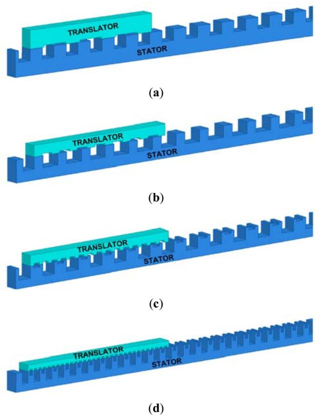
**Figure 1.** Structural details (a) 6/4 LSRM, (b) 6/8 LSRM, (c) Proposed 6/16 LSRM and (d) 12/32LSRM.
