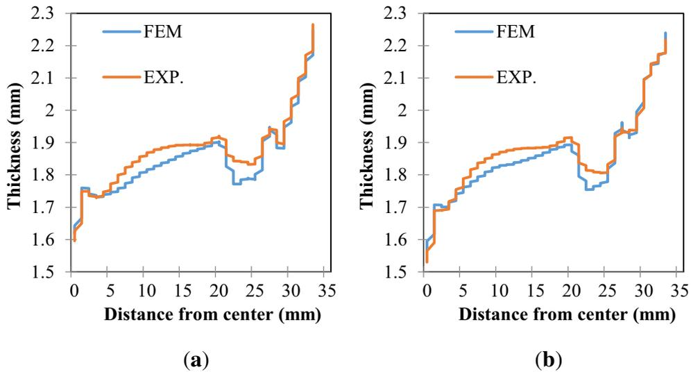
**Figure 4.** Comparison of thickness for (a) hydrodynamic deep drawing process for  $P = 5$  MPa,  $FC = 0.08$ , and  $R = 3$  mm, (b) hydromechanical deep drawing process for  $P = 5$  MPa,  $FC = 0.08$ ,  $R = 3$  mm, and  $F = 20$  kN.
