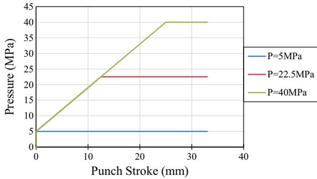
**Figure 2.** The applied internal pressure in the die set.
