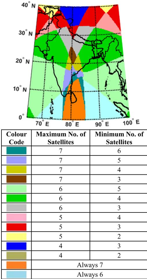
**Figure 4.** NavIC visibility over primary service region with 30° elevation mask for a day
