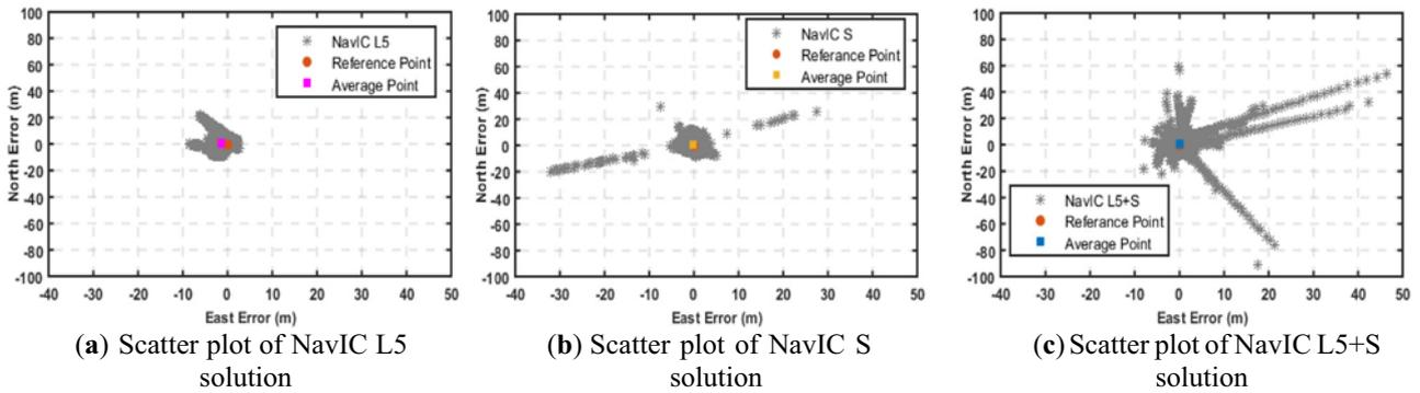
**Figure 7.** (a) Scatter plot of NavIC L5 solution. (b) Scatter plot of NavIC S solution. (c) Scatter plot of NavIC L5+S solution
