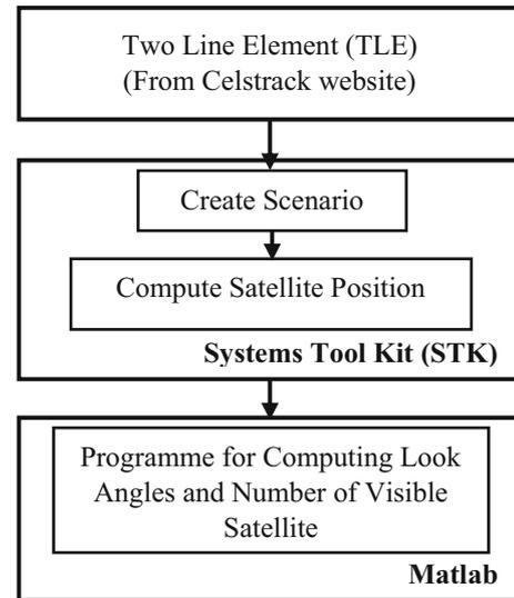
**Figure 1.** Block diagram of NavIC visibility prediction simulation tool
