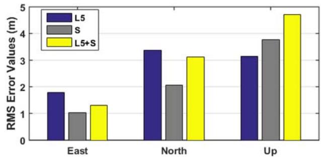
**Figure 6.** Single point solution (SPS) components in East, North and Up directions in NavIC L5, S and L5+S operation from GLB, Burdwan, February, 2019
