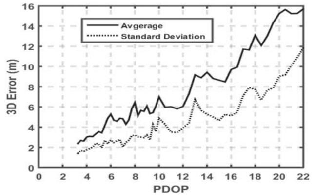
**Figure 5.** Variation of 3d position error with PDOP for NavIC
