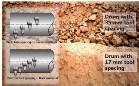
**Figure 12.** Chip size variation for same rock type by altering pick spacing.
