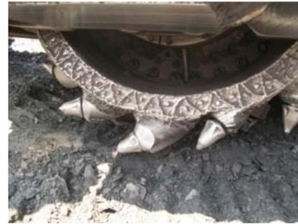
Figure 3. Point attack picks used in SM.
