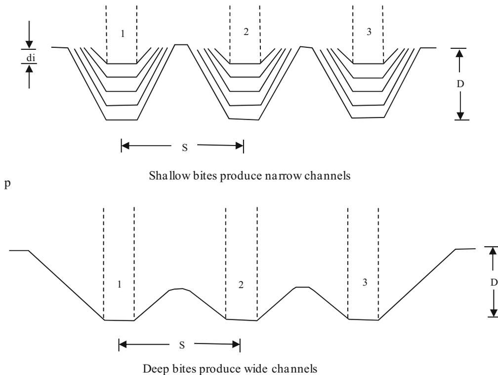
Figure 7. Shallow and deep depth of bites.
