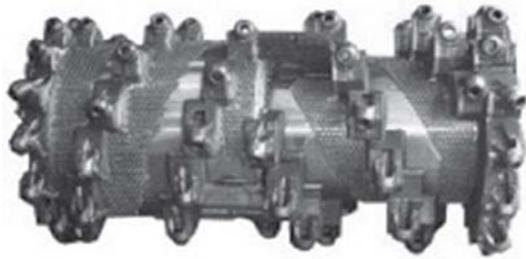
Figure 9. Pick box arrangement of 2200SM SM [16].
