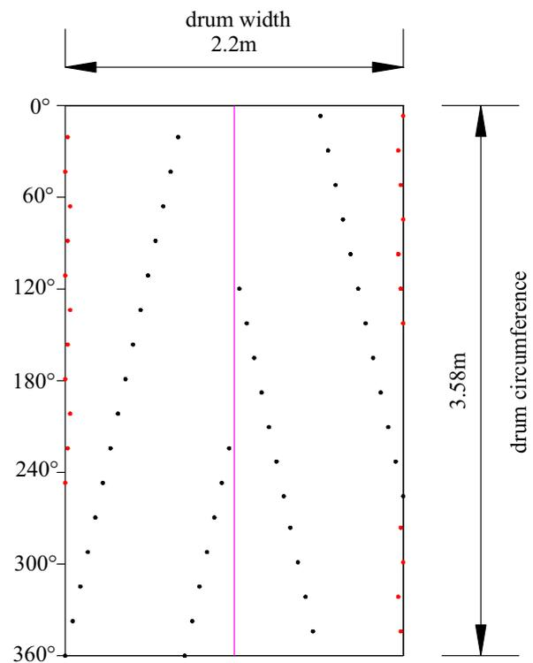
**Figure 11.** Layout of pick arrangement for acquiring 100 mm chip size [18].
