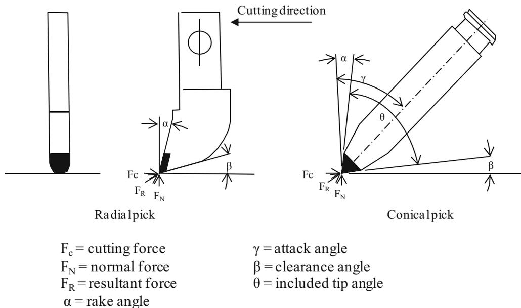
Figure 2. Design of radial and conical pick.
