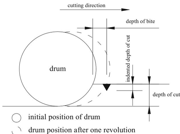
**Figure 1.** Cut parameters of SM drum.
