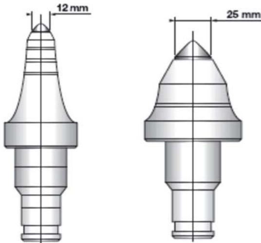
**Figure 5.** Small and large diameter tungsten carbide conical pick.
