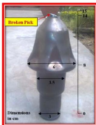
**Figure 6.** Dimension of the pick used in drum design.
