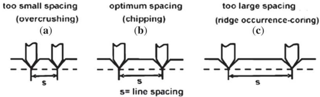
Figure 8. Pick spacing with indented depth of cut.
