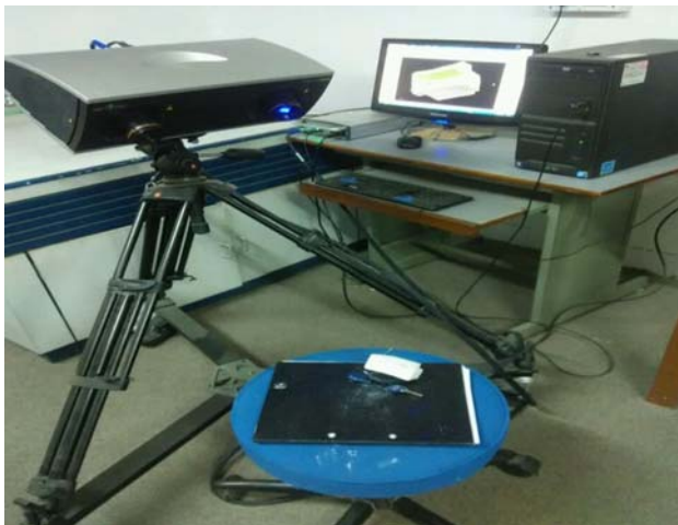
Figure 7. Steinbichler Comet L3D during scanning
