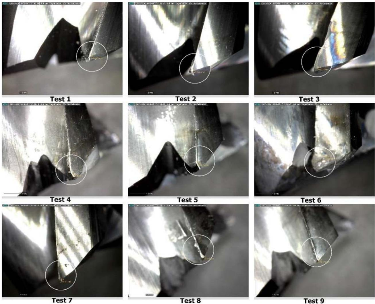
**Figure 7.** Wear images obtained from digital microscope.
