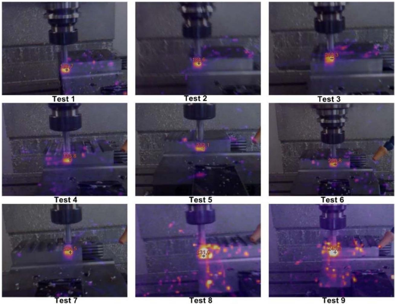
**Figure 6.** Images on temperatures measured in experiments.
