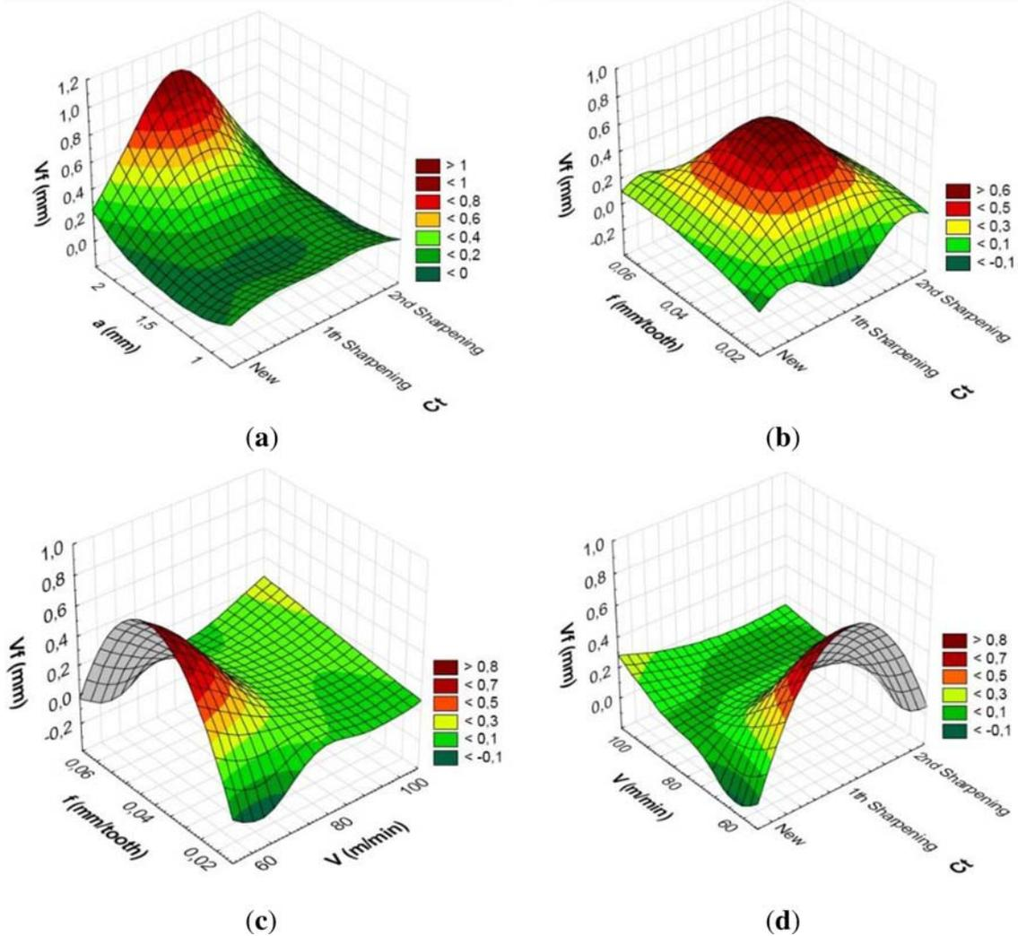
Figure 5. Cutting parameters and tool wear graphs.
