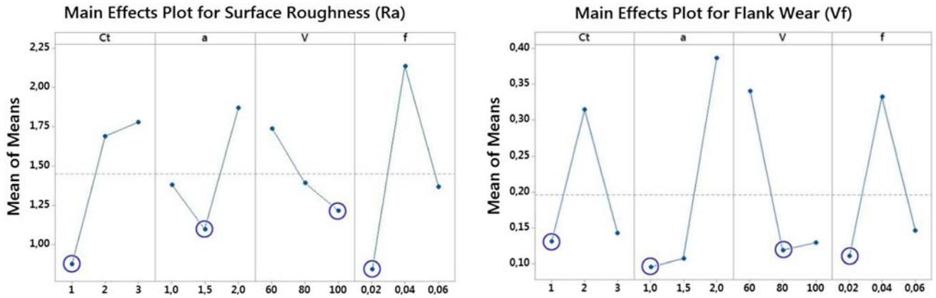
Figure 3. Effect plots of cutting parameters for surface roughness and wear.
