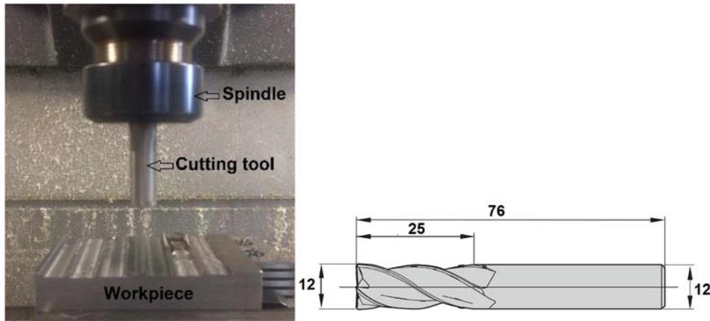
**Figure 1.** Experimental set-up and cutting tool dimensions.
