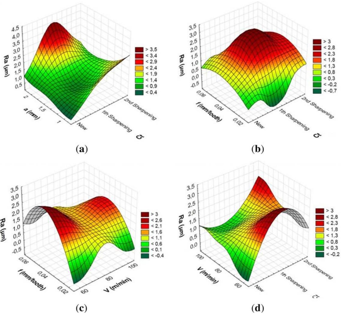
Figure 4. Cutting parameters and surface roughness graphs.
