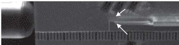
**Figure 11.** Image during crack growth in P-E-P plate.
