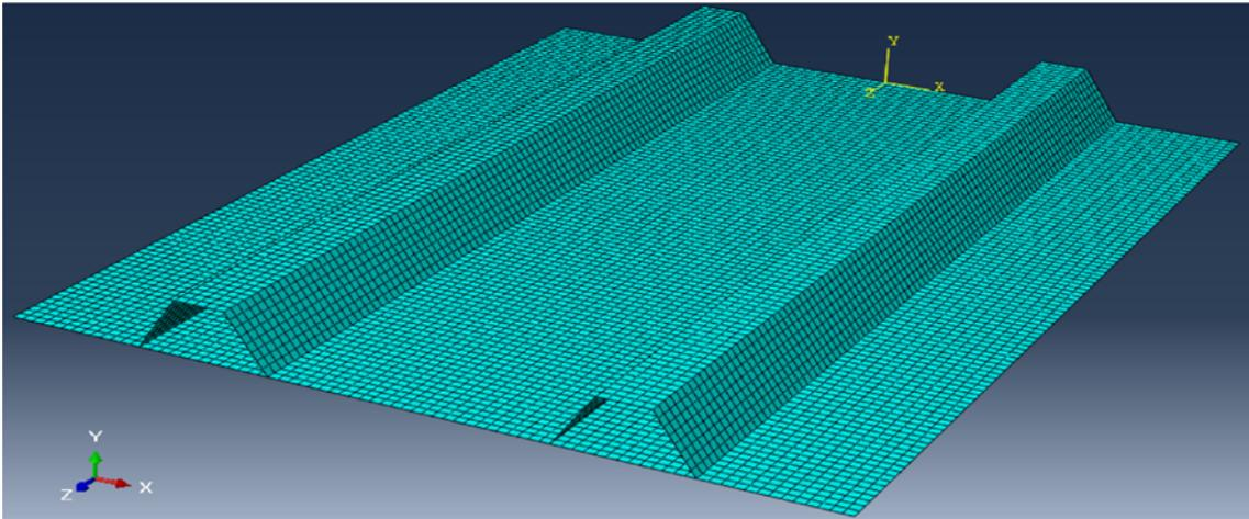
**Figure 12.** The panel discretized with shell element (S4R).
