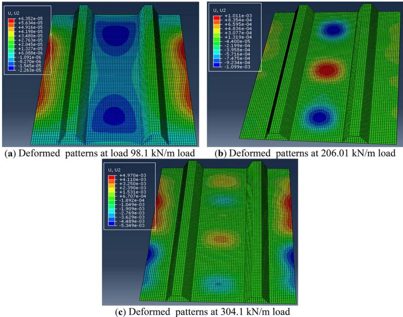
**Figure 14.** The out of plane displacement pattern at different load for FE analysis.
