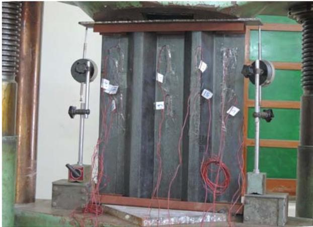
Figure 4. Specimen of hat-stiffened panel installation.
