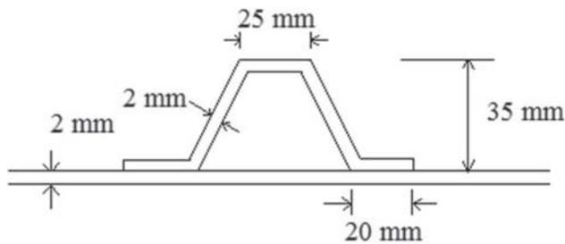
Figure 2. Cross section of the hat-stiffener with plate.
