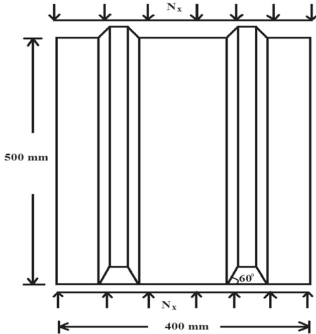
Figure 1. The structural geometry of the hat-stiffened panel.
