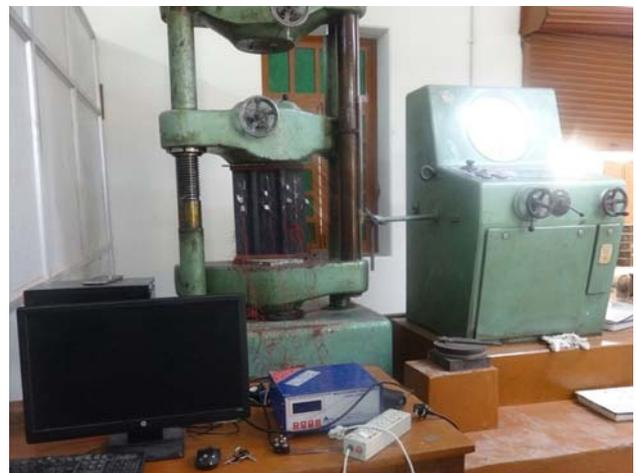
Figure 3. Experimental set-up of hydraulic machine with strain gauge data-logger system.
