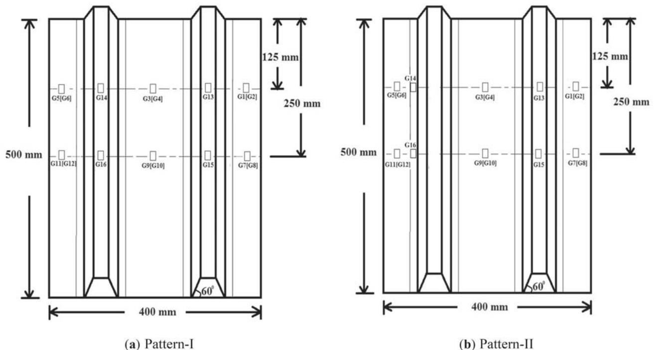
Figure 5. Locations of the strain gauges on panel.
