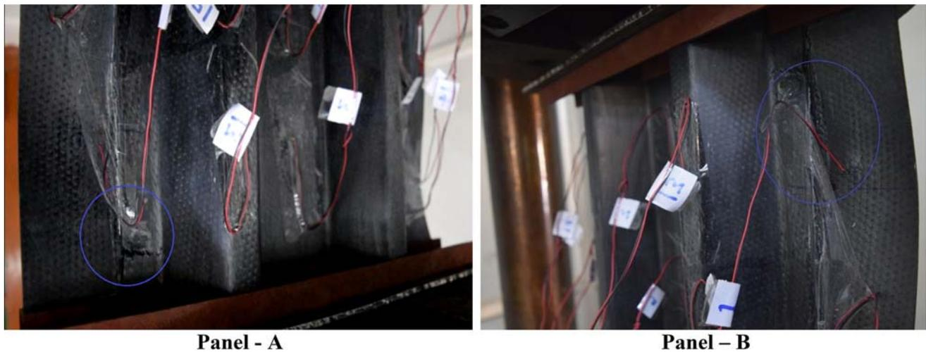
**Figure 6.** Failure mode of the panel.
