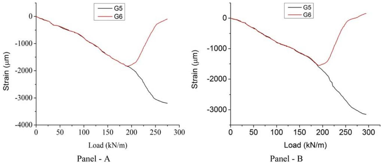
Figure 10. Strain-load curves of strain gauge G5 and G6.
