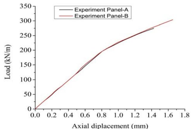
**Figure 7.** Load – axial displacement curves of experimental panel.
