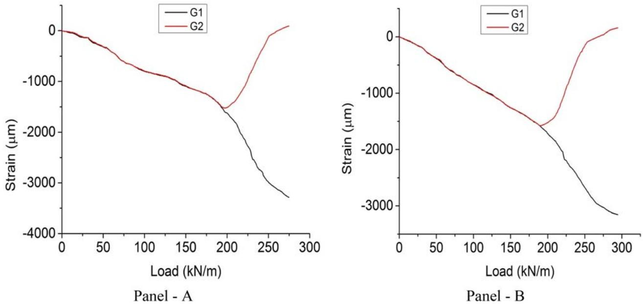
**Figure 8.** Strain-load curves of strain gauge G1 and G2.
