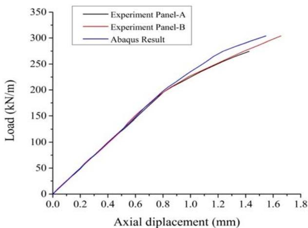
**Figure 13.** Load–axial displacement curves of experimental and simulated panel.
