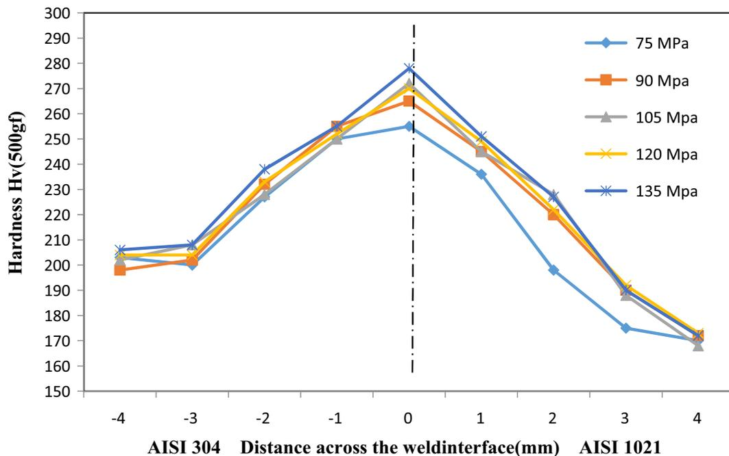
**Figure 8.** Variation of hardness across the weld interface for friction welded AISI 304 and AISI 1021 steel samples subjected to micro hardness testing.
