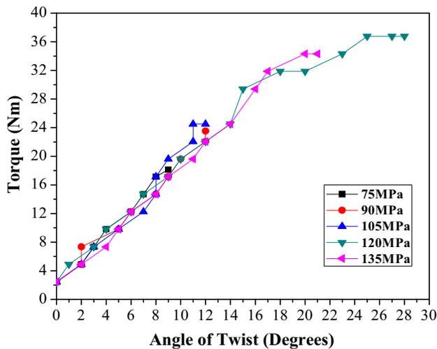
**Figure 6.** Relationship between torque and angle of twist for friction welded AISI 304 and AISI 1021 steel samples subjected to torsion tests.
