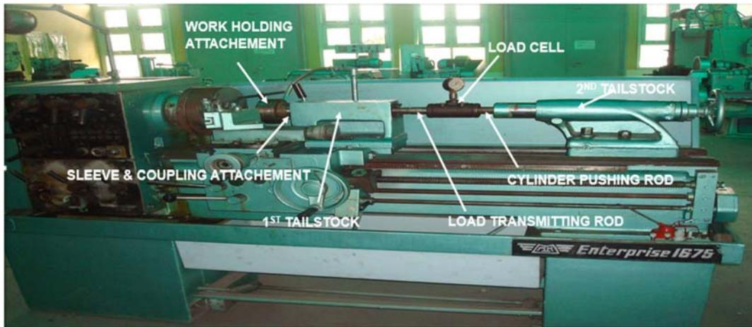
**Figure 1.** Custom made friction welding set-up.
