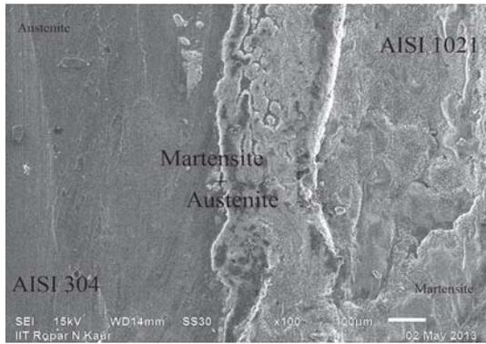
**Figure 9.** Depicts the formation of martensite and highly compressed zone at the weld interface.
