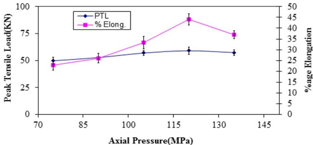
**Figure 5.** Relationship between average peak tensile load and %age elongation for friction welded AISI 304 and AISI 1021 steel samples subjected to tensile tests.
