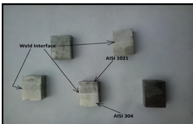
**Figure 2.** Produced samples from cylindrical weldments used for hot corrosion study.
