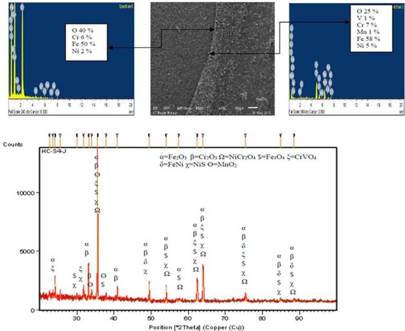
**Figure 12.** SEM/EDS and XRD analysis of AISI 304 and AISI 1021 steel weldments prepared at 1430 rpm at an axial pressure of 120 MPa.
