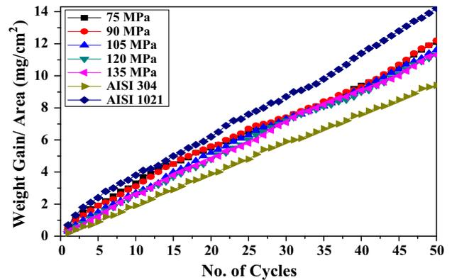
**Figure 11.** Cumulative weight gain graph of both the parent metals as well as friction welded samples prepared at different axial pressures.
