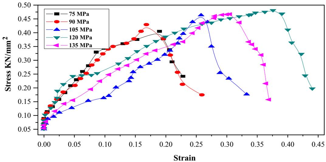
**Figure 3.** Relationship between stress and strain for friction welded AISI 304 and AISI 1021 steel samples.
