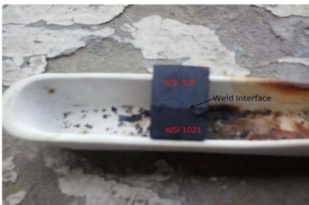
**Figure 10.** Macrograph of a friction welded AISI 304 and AISI 1021 steel sample, prepared at 1430 rpm and 120 MPa axial pressure, subjected to hot corrosion testing in  $\text{Na}_2\text{SO}_4 + \text{V}_2\text{O}_5$  60% environment for 50 cycles at 650°C.
