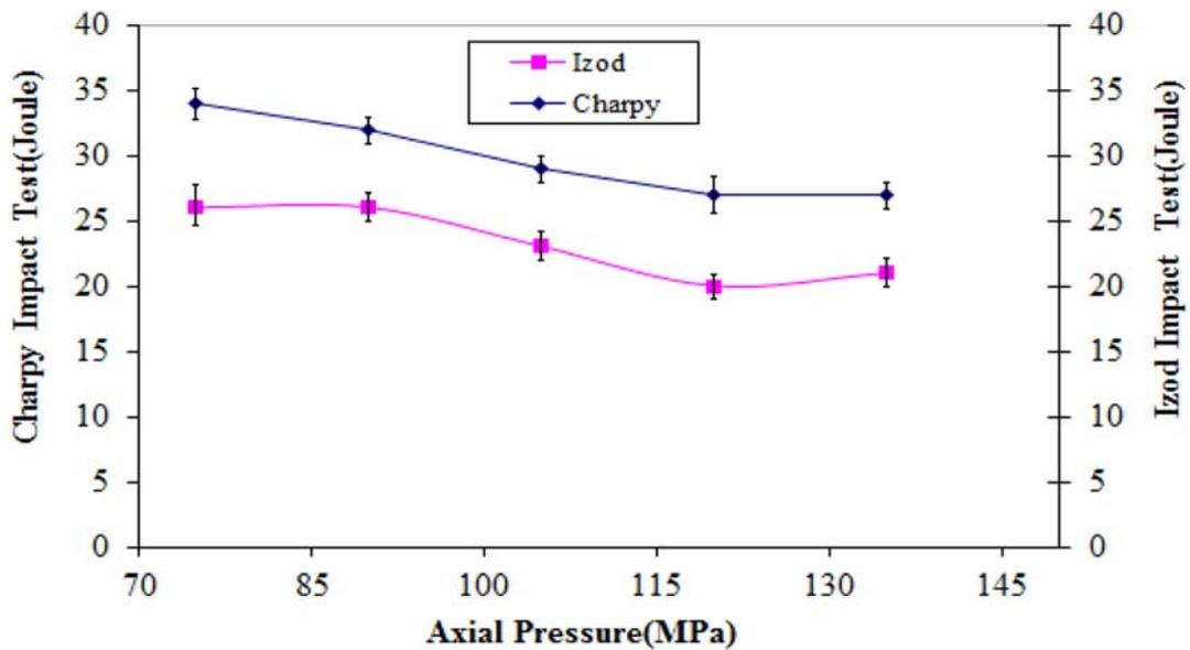
**Figure 7.** Relationship between average impact toughness and axial pressure for friction welded AISI 304 and AISI 1021 steel samples subjected to impact tests.
