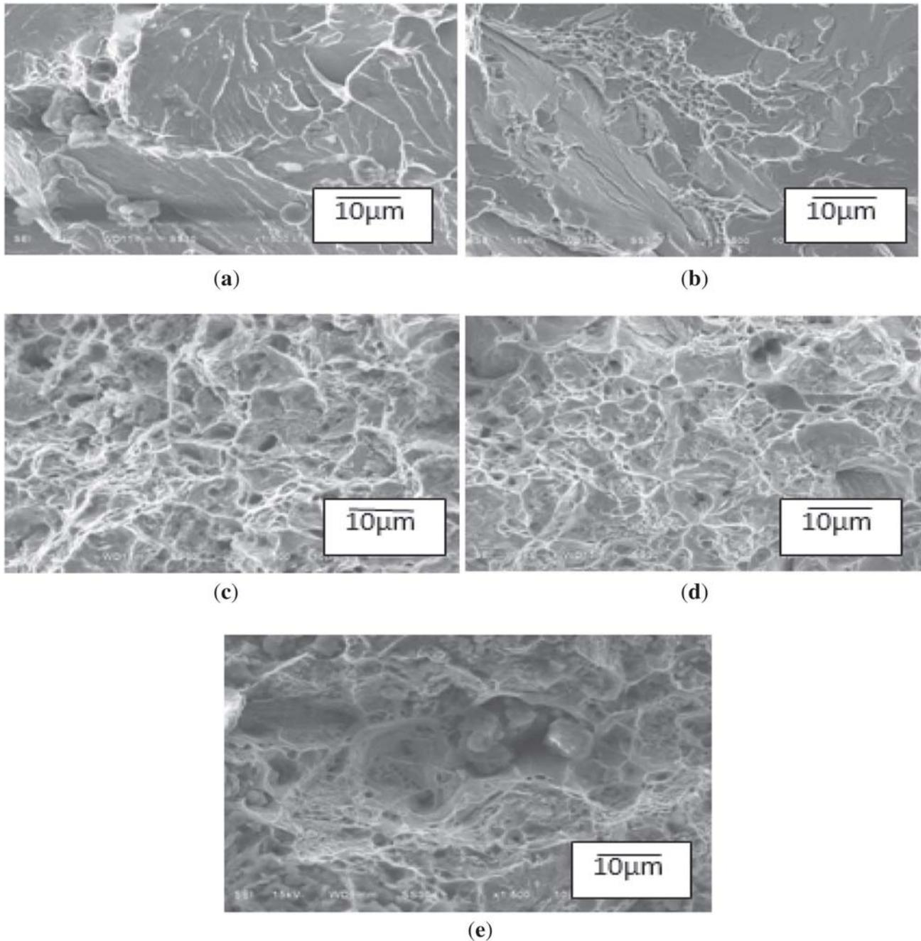
**Figure 4.** SEM fractographs of friction welded AISI 304 and AISI 1021 steel samples failed under tensile testing. The samples were prepared at several axial pressures (a) 75 MPa, (b) 90 MPa, (c) 105 MPa, (d) 120 MPa and (e) 135 MPa.
