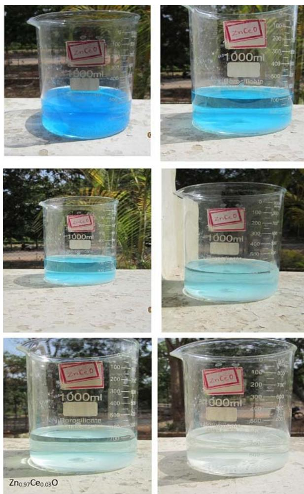
Figure 13. Color change in the MB solution by Ce (x = 0.03 wt%) doped ZnO nanoparticles after exposure to sunlight.
