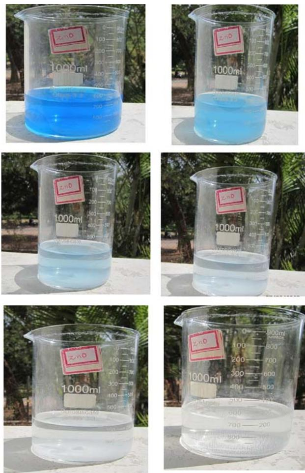
**Figure 10.** Color change in the MB solution by undoped Zinc Oxide nanoparticles after exposure to sunlight.
