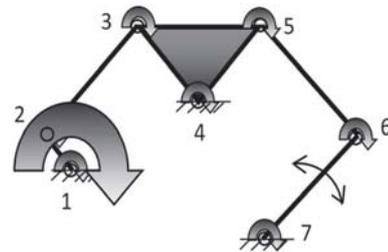
Figure 4. Watt mechanism.
