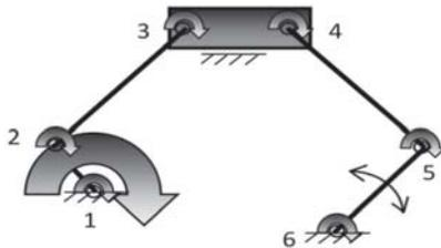
Figure 6. Watt mechanism with slider (2).
