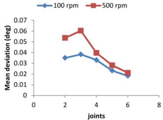
Figure 16. Watt mechanism with 0.1 mm clearance.
