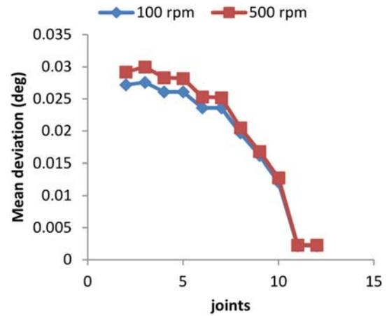
Figure 24. Ten-bar mechanism with 0.1 mm clearance.
