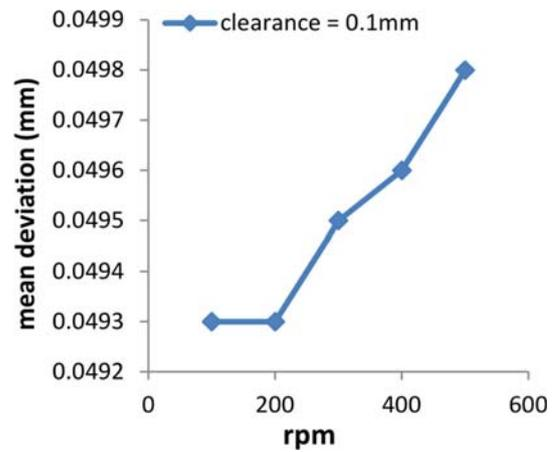
Figure 25. Slider-crank mechanism, Joint 2 deviation v/s speed.
