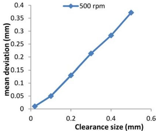
**Figure 27.** Slider-crank mechanism, Joint 2 deviation v/s clearance size.
