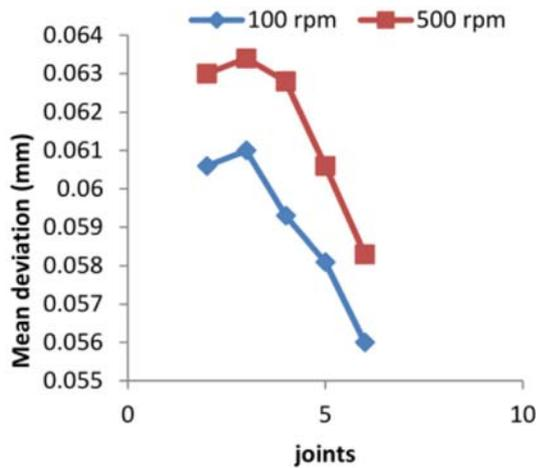
**Figure 17.** Watt mechanism with a slider (1) and 0.1 mm clearance.
