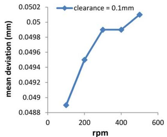
Figure 26. Slider-crank mechanism, Joint 3 deviation v/s speed.
