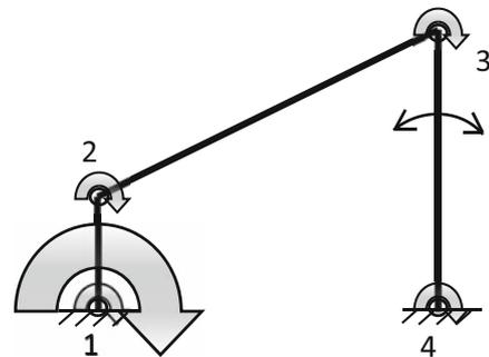
Figure 3. Crank-rocker mechanism.
