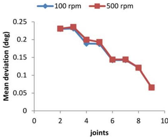
Figure 23. Eight-bar mechanism with 0.1 mm clearance.
