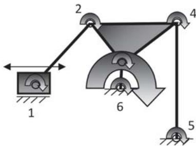
Figure 8. Stephenson1 mechanism with slider.
