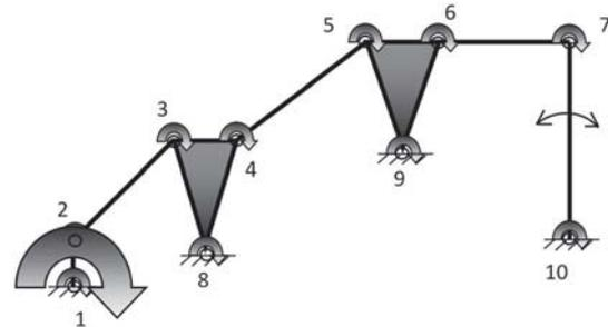
Figure 11. Eight-bar mechanism.
