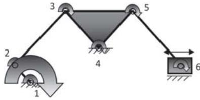
Figure 5. Watt mechanism with slider (1).
