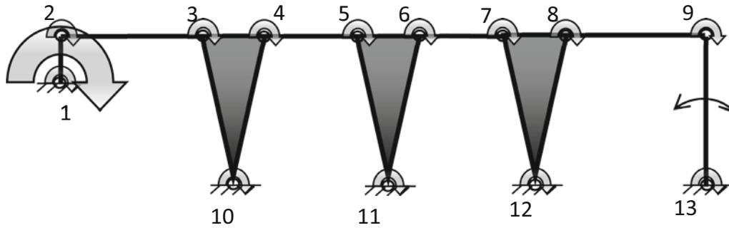
Figure 12. Ten-bar mechanism.
