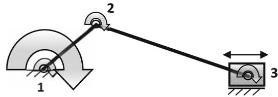
Figure 2. Slider-crank mechanism.
