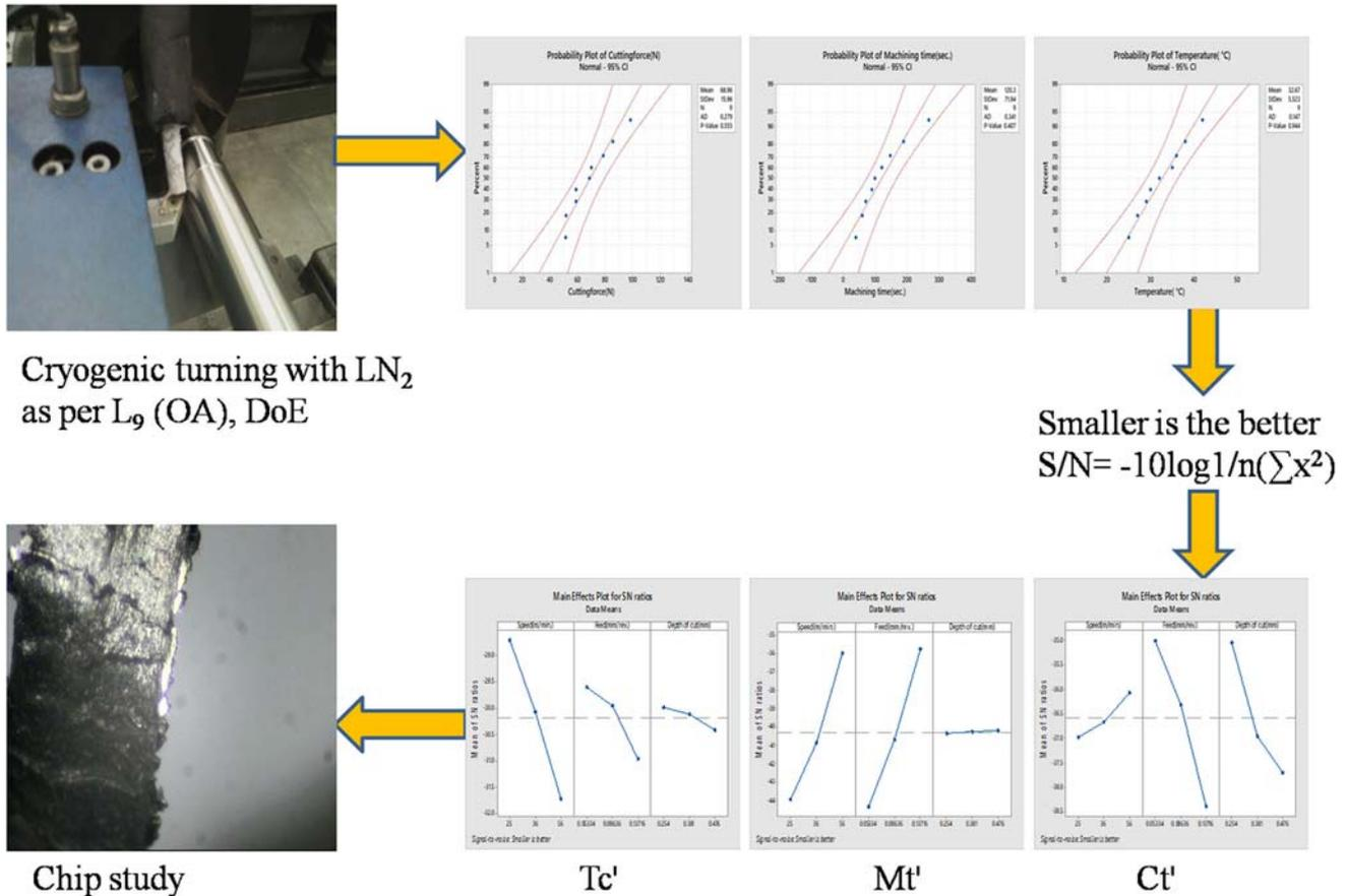
Figure 1. Workflow diagram during turning with LN<sub>2</sub>.
