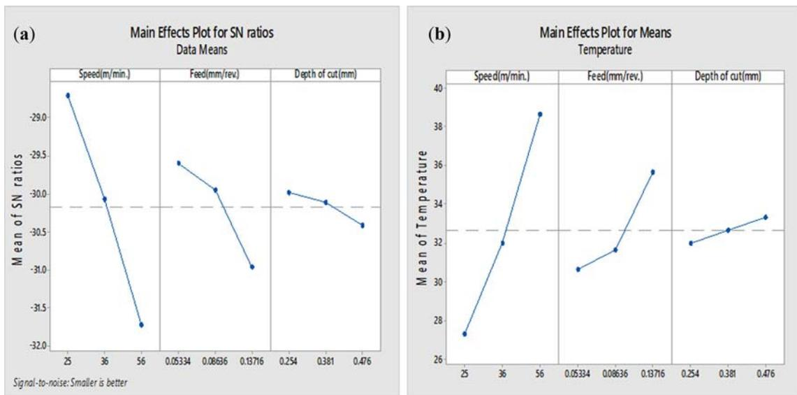
Figure 5. (a) Variation of mean S/N ratio  $Tc'$ . (b) Variation of mean  $Tc'$  with different factor levels.
