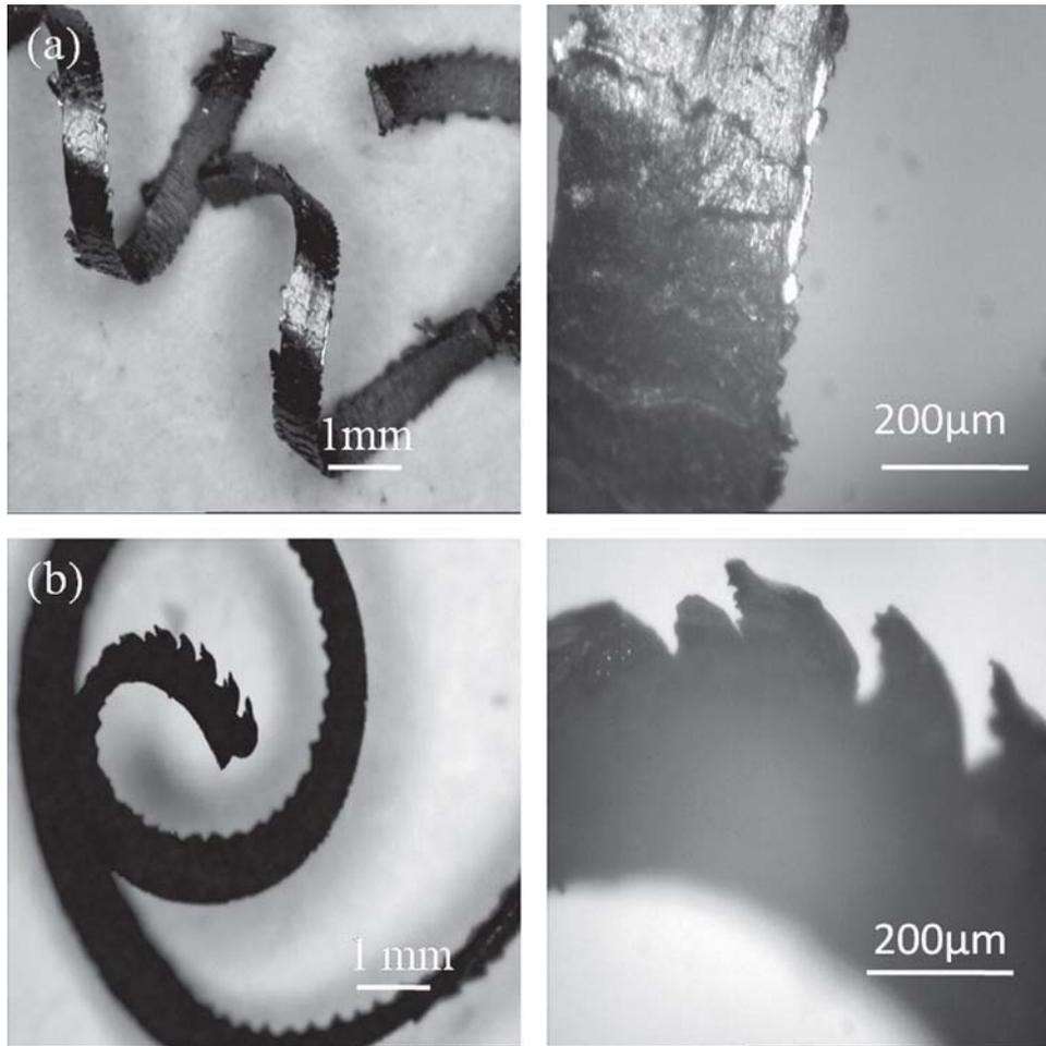
**Figure 7.** (a) Optical images of chip at  $Vd'$  25 m/min.,  $Fd'$  0.05334 mm/rev. and  $Dt'$  0.254 mm. (b)  $Vd'$  56 m/min.,  $Fd'$  0.13716 mm/rev. and  $Dt'$  0.381 mm.
