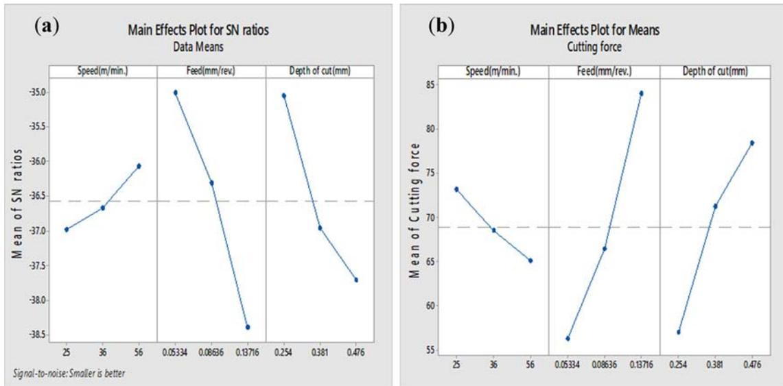
**Figure 3.** (a) Variation of mean S/N ratio  $Ct'$ . (b) Variation of mean  $Ct'$  with different factor levels.
