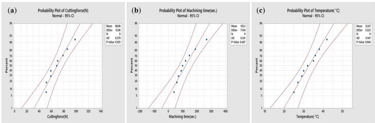
**Figure 2.** Probability plots for (a) cutting force, (b) machining time and (c) temperature.
