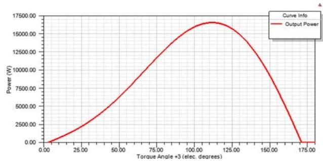
Figure 9. Output Power and Torque Angle Characteristics
