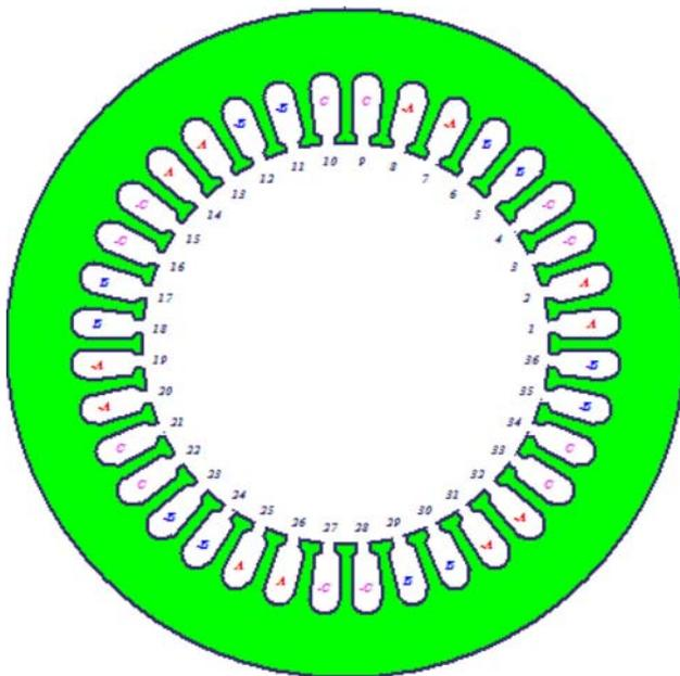
Figure 2. Stator winding layout.
