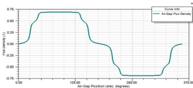
Figure 6. Flux Density in Air gap
