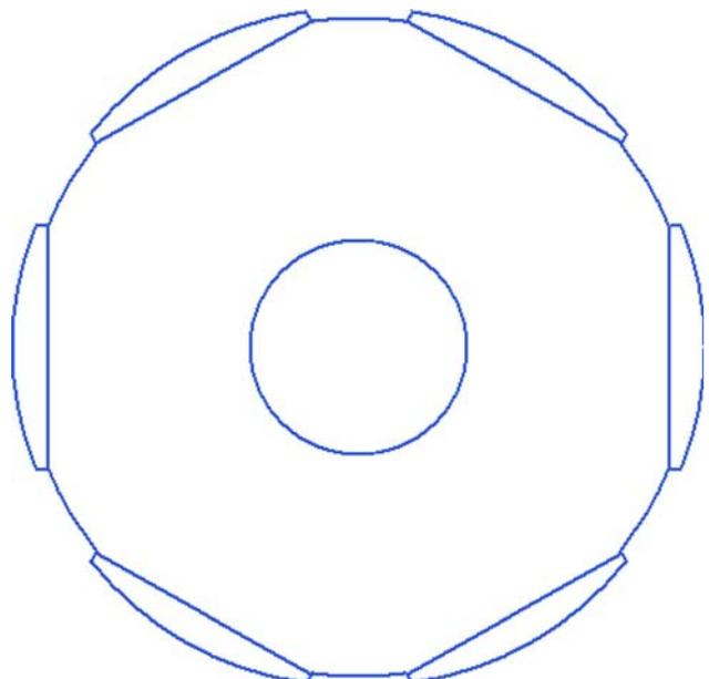
Figure 3. Surface Mounted Magnet Rotor
