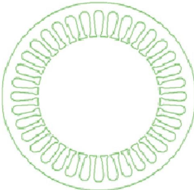
Figure 1. Stator with semi-enclosed slot.
