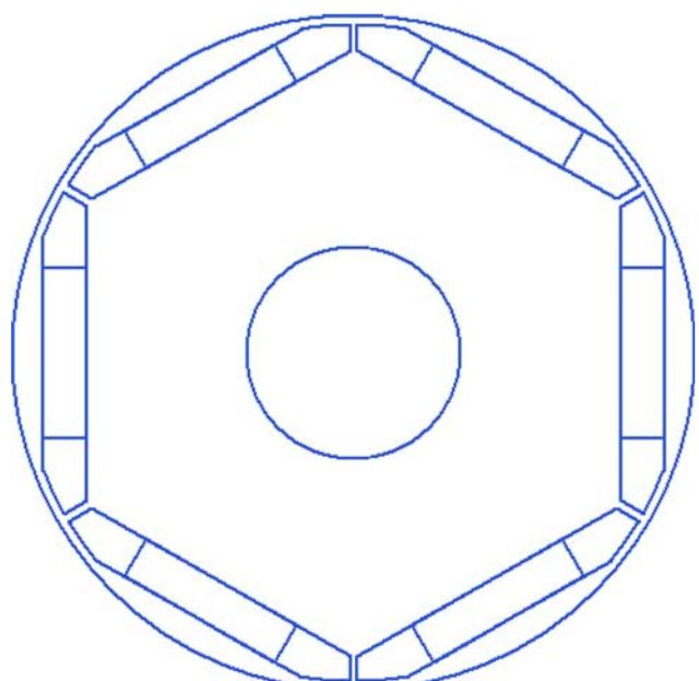
Figure 4. Bridge Type Magnet Rotor
