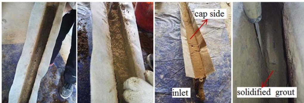
Figure 4. Experiment procedure and excavation results of the grout fracture.
