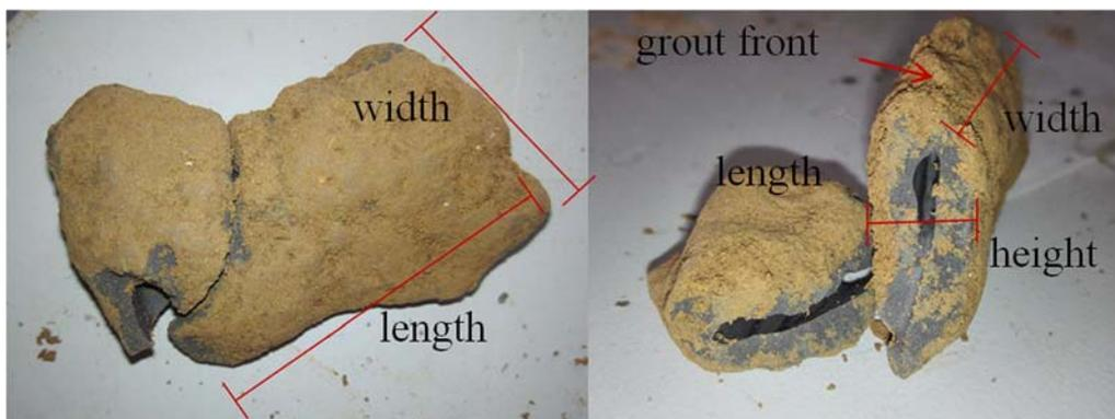
**Figure 6.** Solidified grout after excavation.
