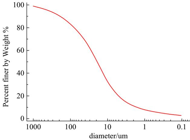
Figure 3. Grain size distribution of the soil medium.
