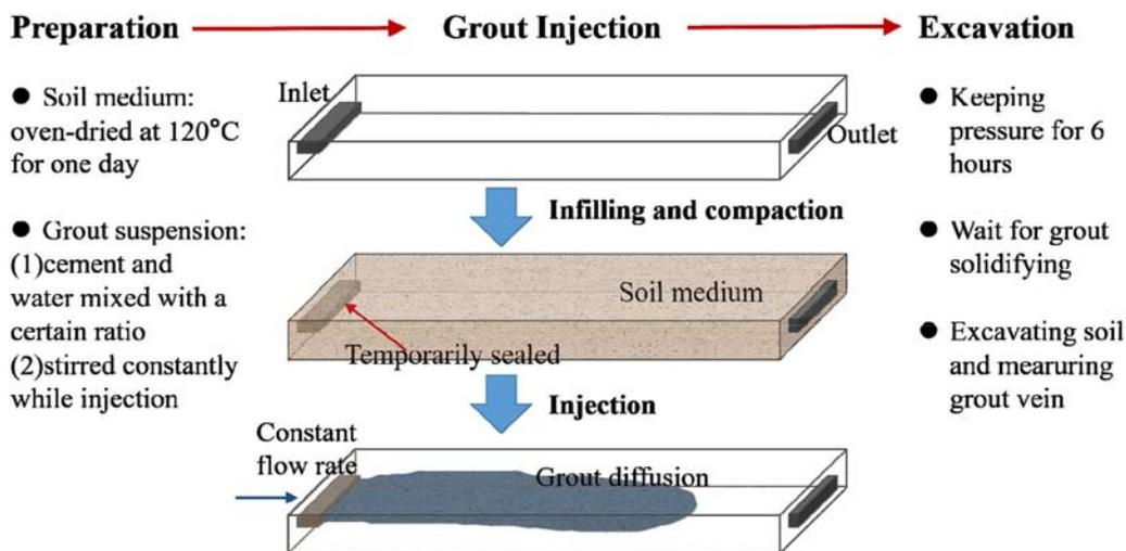
Figure 2. General procedures for the experiment of hydraulic fracturing with grout suspension.
