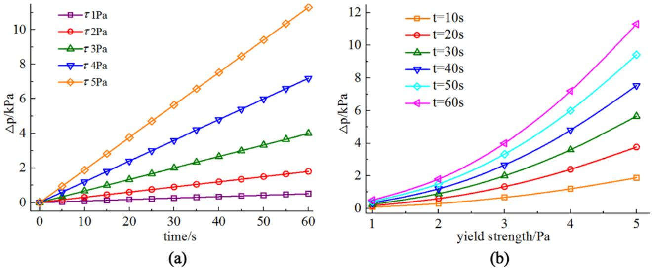
Figure 7. Variation of grout pressure with different times and yield strength.
