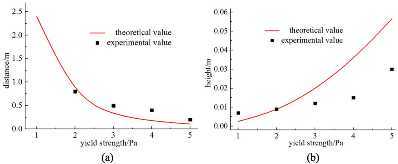
**Figure 5.** Variation of grout distance and grout height with different yield strength.
