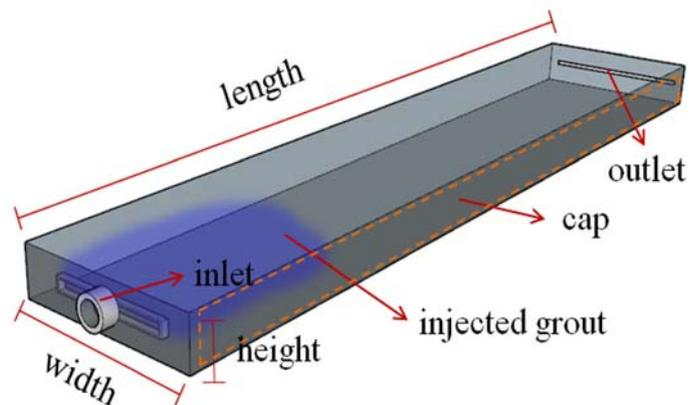
**Figure 1.** Theoretical model of fracture grouting and the flowing pattern in the container of the experiment.
