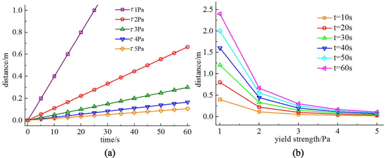
Figure 8. Variation of grouting distance with different times and yield strength.
