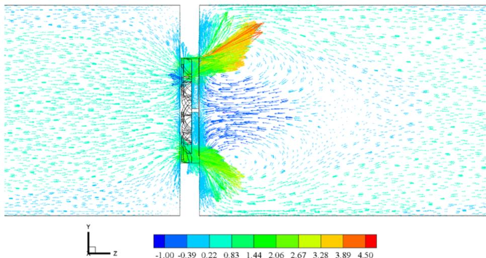
**Figure 4.** Vectors of axial velocity (m/s) in a longitudinal plane shown close to the fan. Volumetric flow rate = 11.5 lpm and pressure rise = 8.03 Pa. Notice the large reversed flow region (with negative velocity) behind the fan. The chemical sensor should *not* be positioned here.
