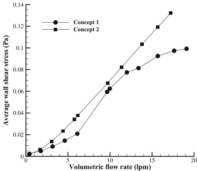
**Figure 7.** Average values of wall shear stress on the disc where the chemical sensor is to be fixed for the two concepts.
