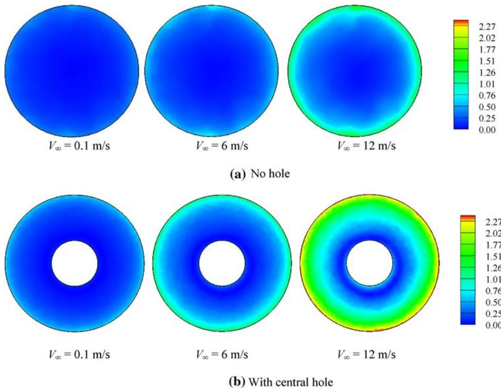
**Figure 21.** Contours of wall shear stress (Pa) on the sensor disc for different freestream velocities for (a) no hole and (b) with central hole on the sensor disc. The angle of attack is  $45^\circ$  in all these cases.
