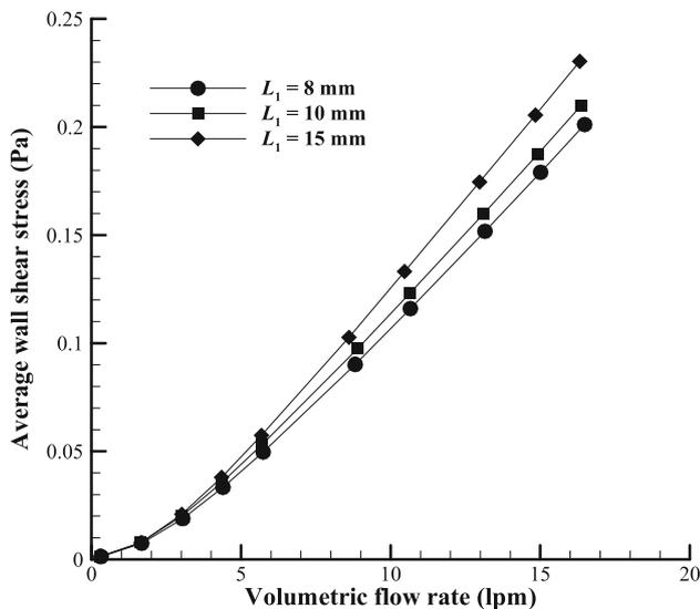
**Figure 13.** Average wall shear stress on the disc for different lengths of converging section  $L_1$ .
