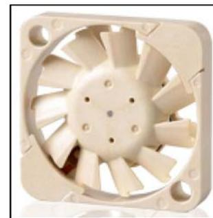
**Figure 1.** Sunon model UF3H3 miniature axial flow fan ([www.sunon.com](http://www.sunon.com)). The fan rotor diameter is 16 mm and the casing size is 17 × 17 × 3 mm.
