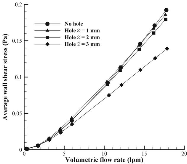
**Figure 9.** Average wall shear stress on the disc for different hole diameters.
