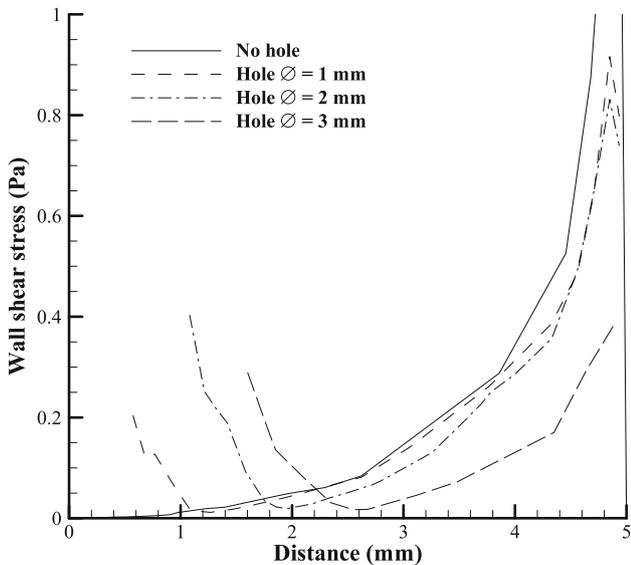
**Figure 10.** Shear stress distribution on the disc in the radial direction.
