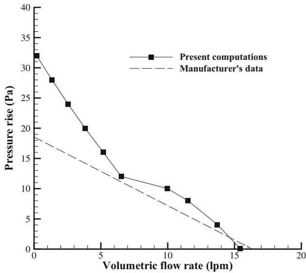
**Figure 3.** Sunon UF3H3 fan computational performance compared with manufacturer data. The fan speed is 13,000 rpm.
