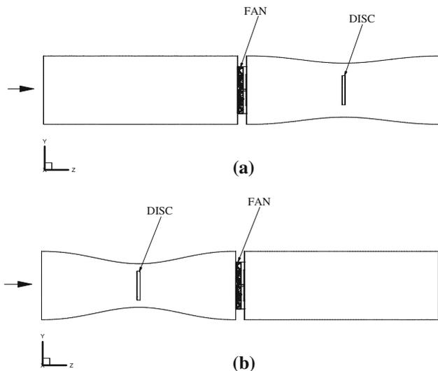
**Figure 5.** Two concepts developed for placing the sensor disc. (a) Concept 1 where the sensor disc is located behind the fan. (b) Concept 2 where the sensor disc is located ahead of the fan. The flow is from left to right in both the concepts.
