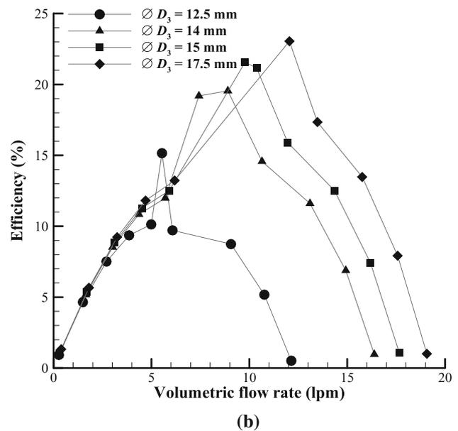
**Figure 11.** Performance of the fan for different throat diameters  $D_3$ . (a) Pressure rise versus fan's flow rate, and (b) hydrodynamic efficiency of the fan.
