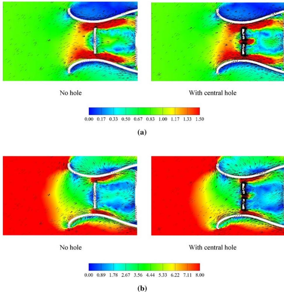
**Figure 22.** Contours of velocity magnitude along with velocity vectors in the vertical azimuthal plane. (a)  $V_\infty = 1$  m/s and (b)  $V_\infty = 12$  m/s. The angle of attack is  $45^\circ$  in all these cases.
