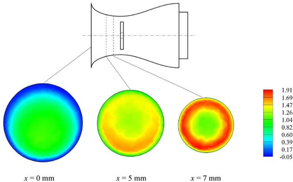
**Figure 20.** Contours of axial velocity (m/s) at various stations in front of the sensor disc. Sensor disc is at  $x = 10$  mm. Forward velocity = 1 m/s and angle of attack =  $45^\circ$ .
