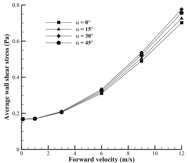
**Figure 19.** Average skin friction on the disc at different forward velocities and angles of attack.
