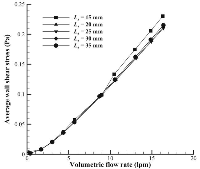
**Figure 14.** Average wall shear stress on the disc for different lengths of diverging section  $L_2$ .
