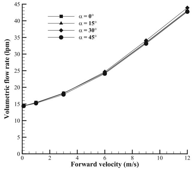
**Figure 18.** Volumetric flow rate at the inlet of air suction duct at different forward velocities and angles of attack.
