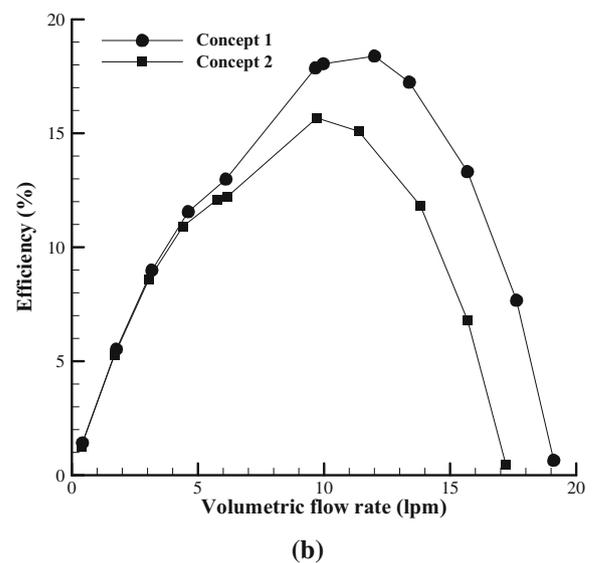
**Figure 6.** Performance of the fan in the two conceptual duct designs. (a) Pressure rise versus fan’s volumetric flow rate along with the system resistance curves and (b) hydrodynamic efficiency of the fan.
