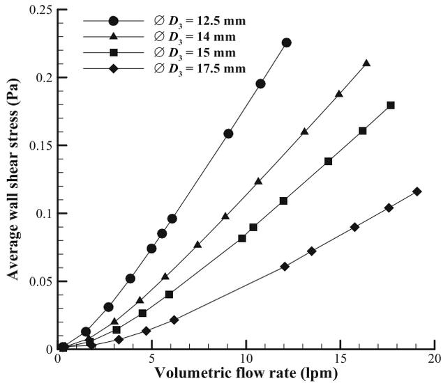
**Figure 12.** Average wall shear stress on the disc for different throat diameters  $D_3$ .
