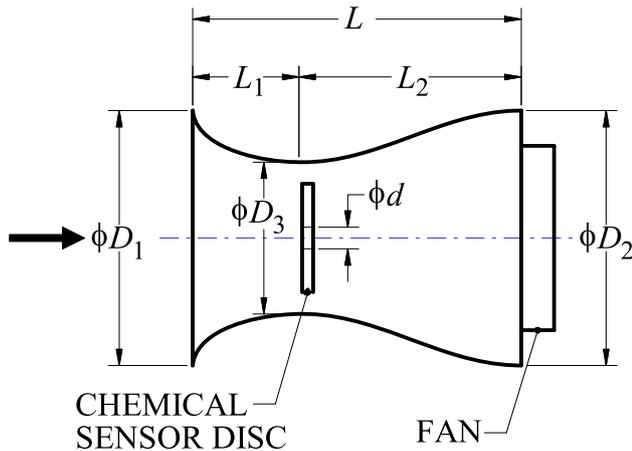
**Figure 15.** Optimised air suction duct design for chemical sensor. The length of the converging section  $L_1 = 10$  mm, the throat diameter  $D_3 = 14$  mm and the length of the diverging section  $L_2 = 20$  mm. The disc with 10 mm diameter has a central hole of  $d = 2$  mm diameter.
