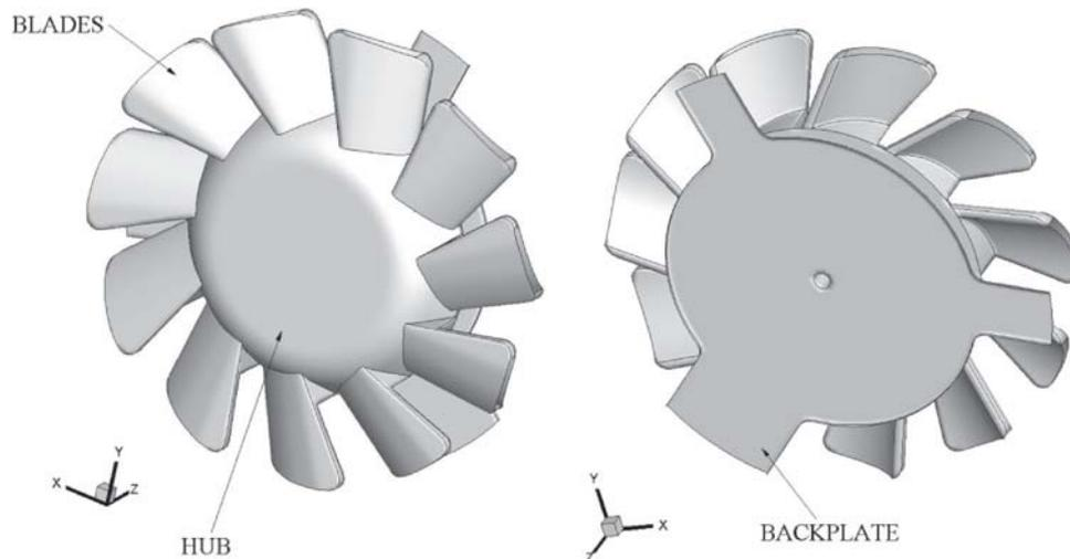
**Figure 2.** Geometry of Sunon UF3H3 fan. The eleven blades can be seen in the figure on the left and the back plate on the right.
