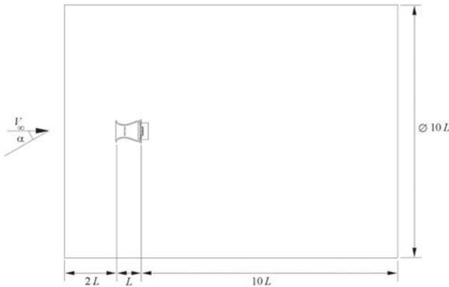
**Figure 17.** Computational domain to study the effect of free-stream velocity and angle of attack.  $L = 30$  mm.
