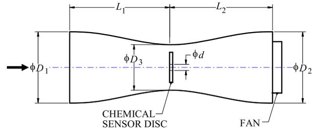
**Figure 8.** Conceptual air suction duct design for chemical sensor.
