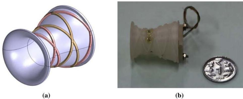
**Figure 16.** (a) Structural design of air suction duct with helical ribs. (b) Air suction duct fabricated by Rapid Prototyping using ABS plastic material.
