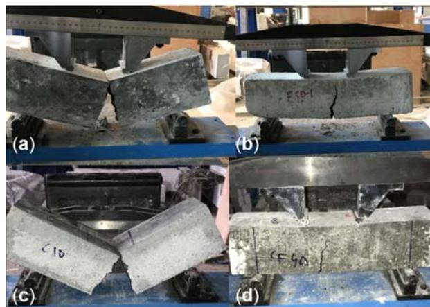
**Figure 6.** Failure modes of unconfined RuC beams with (a) 0% rubber, (b) 50% fine rubber, (c) 10% coarse rubber, and (d) 40% fine and coarse rubber content.
