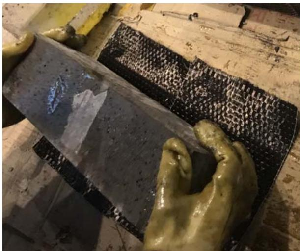
**Figure 4.** Fabrication of FRP jackets.
