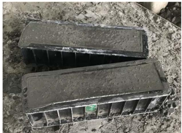
**Figure 3.** Casting of rubberized concrete beams.
