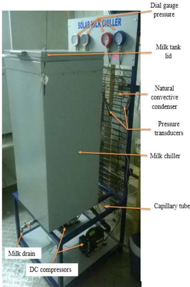
**Figure 3.** Photographic representation of the vertical milk chiller.
