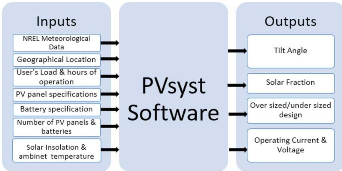
**Figure 1.** Outline of the simulation process using the PVsyst software.
