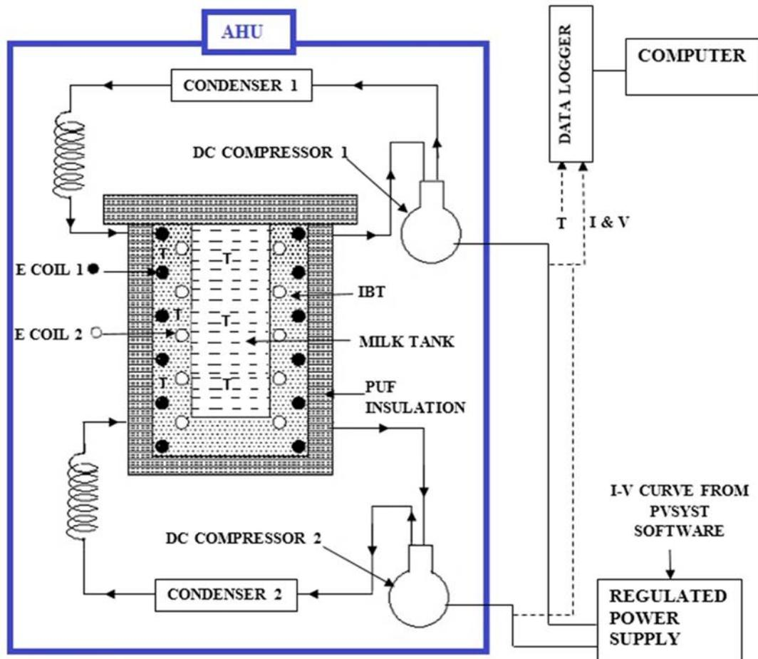
**Figure 2.** Schematic layout of the milk chiller and test facility.
