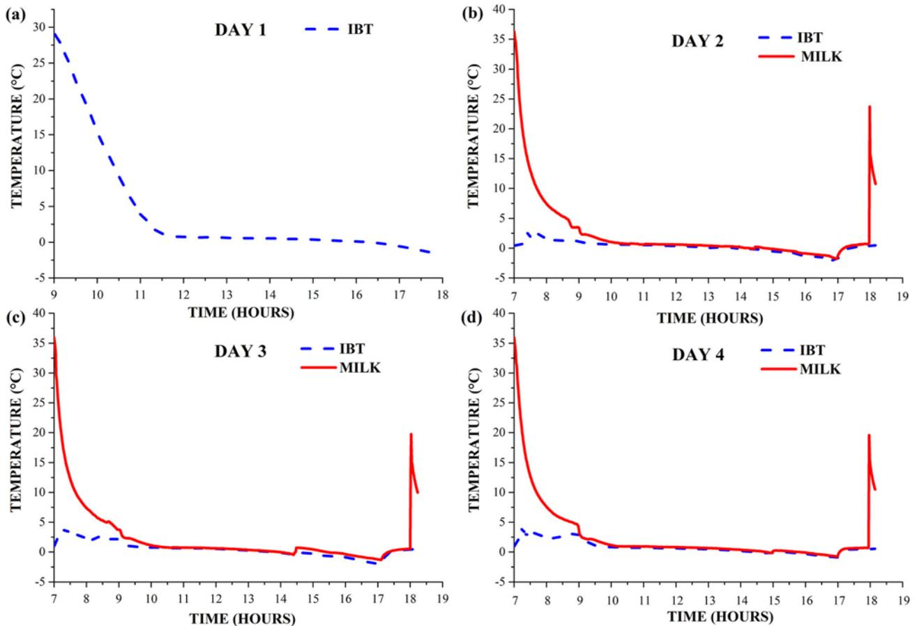
**Figure 5.** Pull down characteristics of the milk chiller day 1 to 4.
