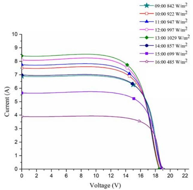
**Figure 4.** Hourly I-V curves for different solar irradiation generated from PVsyst software.
