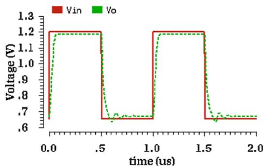
**Figure 9.** Transient response of proposed FVF cell for square input pulse.
