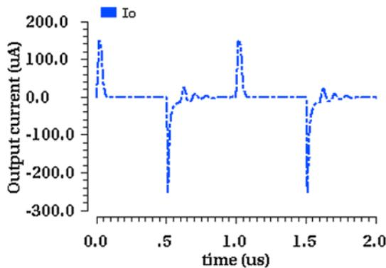
**Figure 10.** Current sourcing and sinking capabilities of proposed FVF cell.
