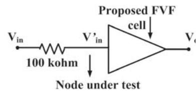
**Figure 12.** Simulation set up to calculate input capacitance.
