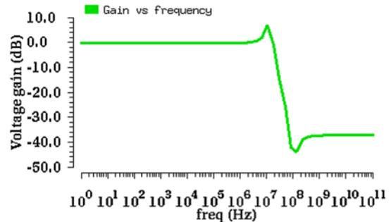
Figure 6. Frequency response of proposed FVF cell.
