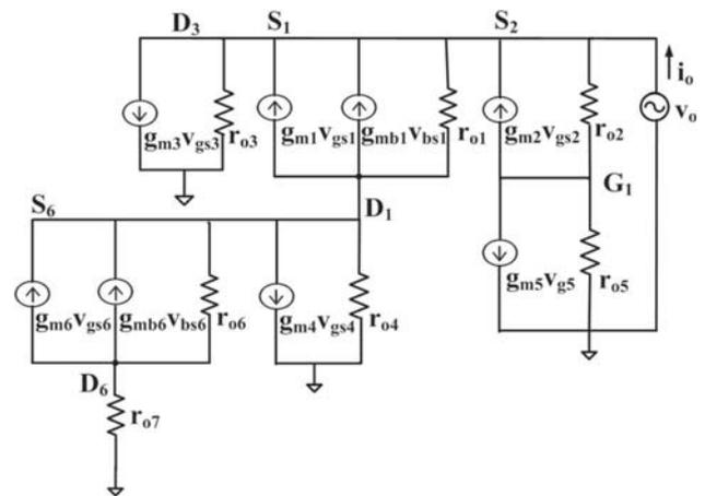
Figure 3. Small-signal equivalent model of proposed FVF cell.
