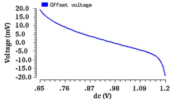
Figure 5. Offset voltage of proposed FVF cell.
