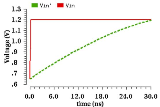
**Figure 13.** Rise time of voltage ( $V'_{in}$ ) at node under test.
