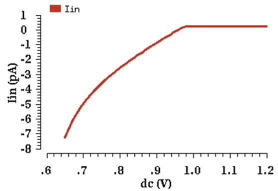
**Figure 11.** Input current of proposed FVF cell.
