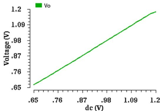
Figure 4. Transfer characteristic of proposed FVF cell.
