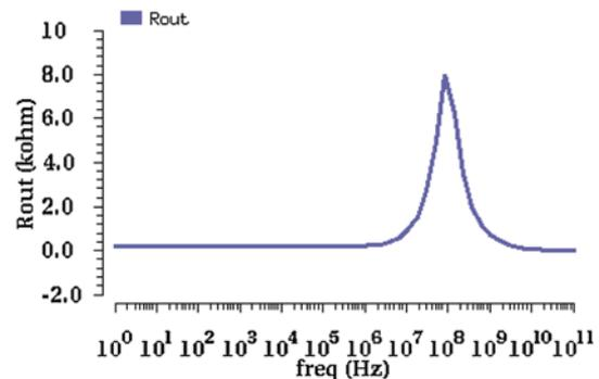
Figure 7. Output resistance of proposed FVF cell.
