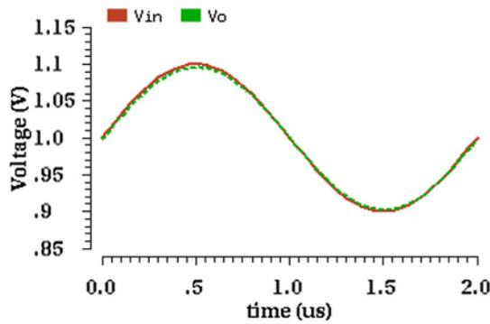
**Figure 8.** Transient response of proposed FVF cell for sinusoidal input voltage.
