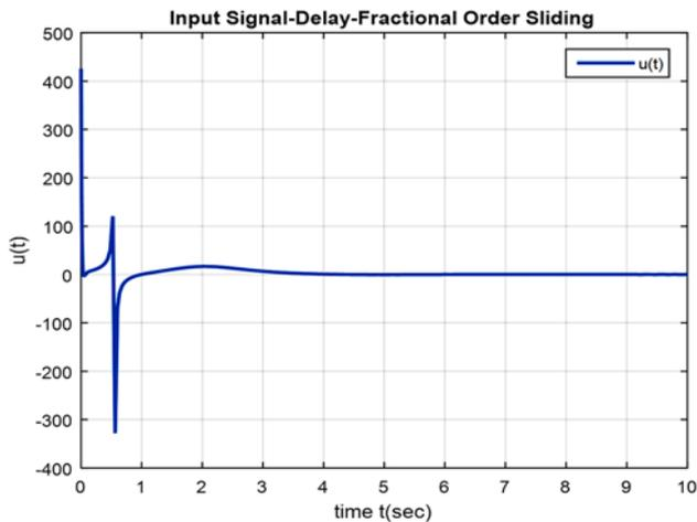
**Figure 5.** The control effort through fractional-order sliding mode control approach under the Smith predictive method for the inverted pendulum system with delay.
