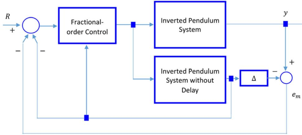
**Figure 2.** The schematic diagram of Smith predictive fractional-order sliding mode control approach with delay.
