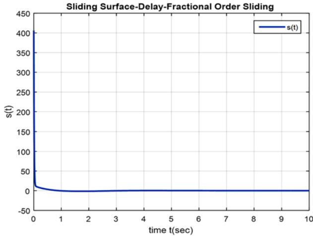
**Figure 4.** The sliding surface through fractional-order sliding mode control approach under the Smith predictive method for the inverted pendulum system with delay.
