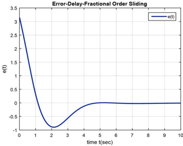
**Figure 3.** The states error through fractional-order sliding mode control approach under the Smith predictive method for the inverted pendulum system with delay.
