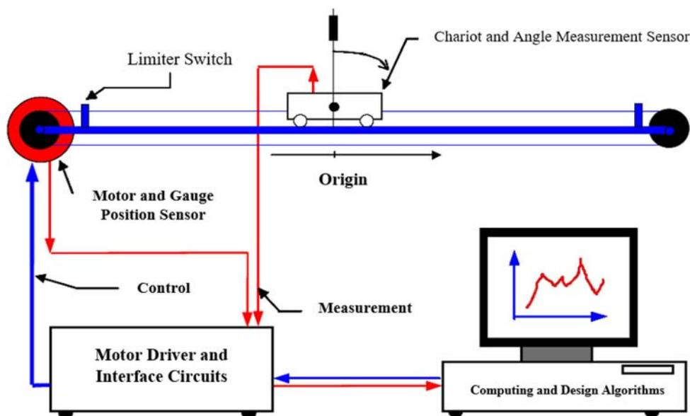
Figure 1. An overview of a laboratory for inverted pendulum system.
