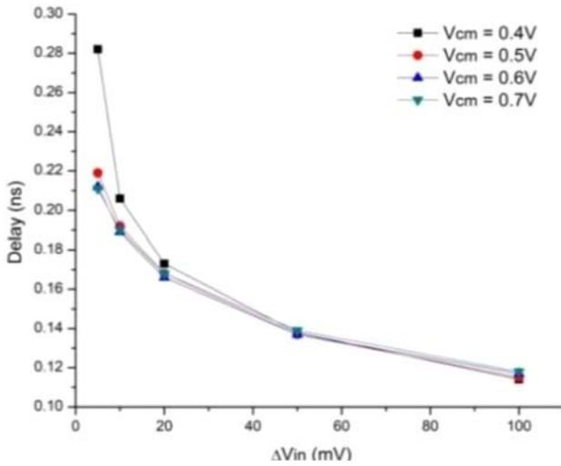
Figure 3. Delay versus input differential voltage ( $\Delta V_{in}$ ).
