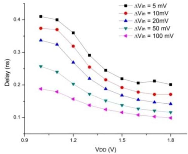
Figure 6. Delay versus supply voltage ( $V_{DD}$ ).
