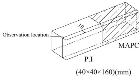
Figure 1. Bonded specimens.
