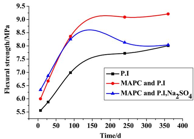
Figure 2. Flexural strength of specimens under different environments.
