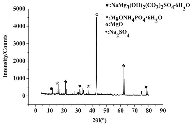
**Figure 6.** XRD of MAPC cross section in  $\text{Na}_2\text{SO}_4$  for 360 days.
