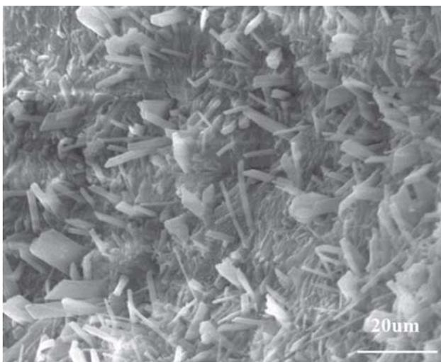
**Figure 7.** SEM of MAPC cross section in  $\text{Na}_2\text{SO}_4$ .
