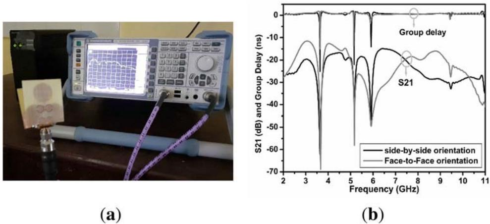
**Figure 8.** (a) Measurement set-up (face to face orientation) and (b) plot of magnitude response of antenna transfer function ( $S_{21}$ ) and group delay (side by side and face to face orientation).
