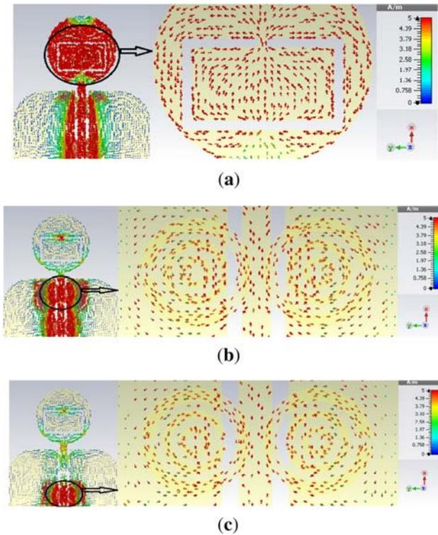
**Figure 5.** Simulated surface current on antenna at (a) 3.62, (b) 5.2 and (c) 5.92 GHz.
