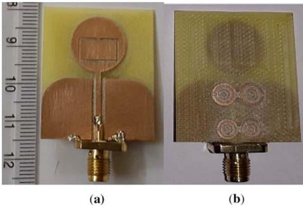
**Figure 3.** Prototype of (a) top and (b) bottom of proposed antenna.
