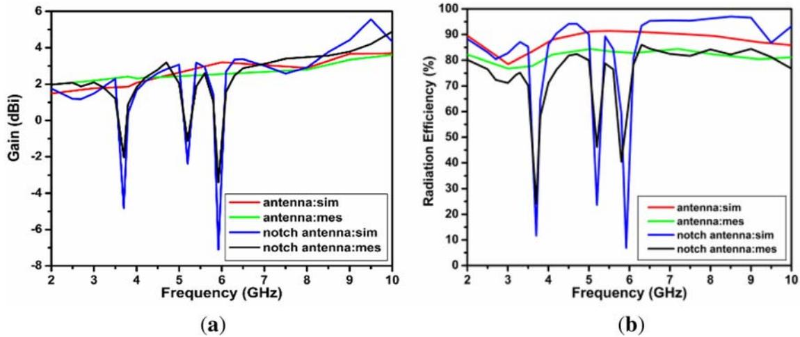
**Figure 7.** Simulated and measured comparison plot for reference antenna and the proposed triple notched antenna of (a) Gain over frequency, (b) radiation efficiency over frequency.
