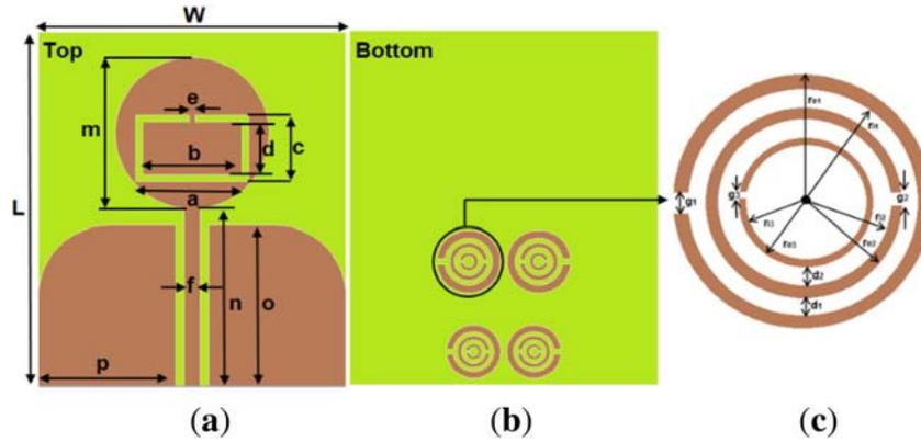
**Figure 1.** Schematics of the proposed antenna: (a) top view, (b) bottom view and (c) three- layered circular SRR.
