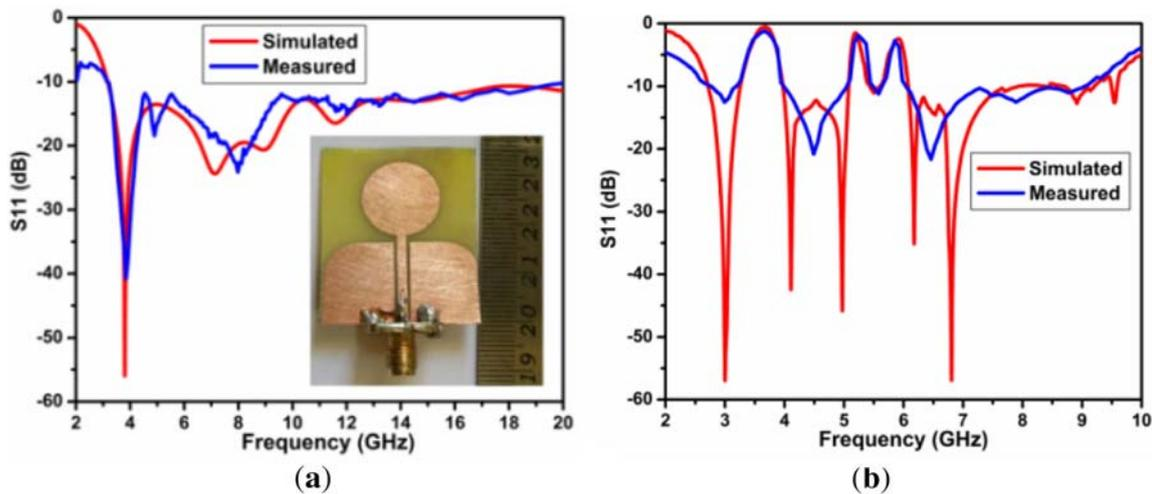
**Figure 4.** Simulated and measured  $S_{11}$  response of (a) reference antenna, (b) proposed triple notched antenna.
