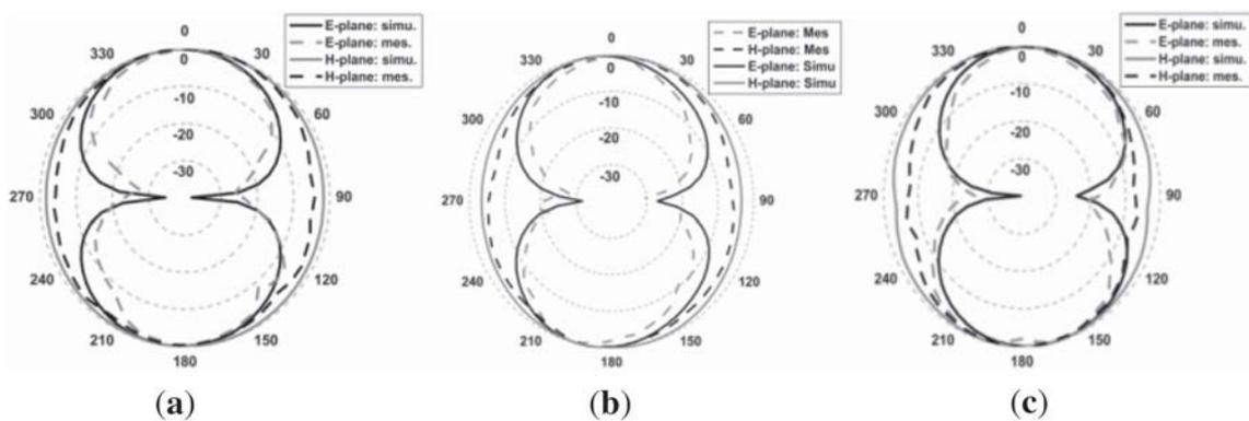
**Figure 6.** E-plane and H-plane antenna radiation patterns at (a) 4.5, (b) 7 and (c) 9 GHz.
