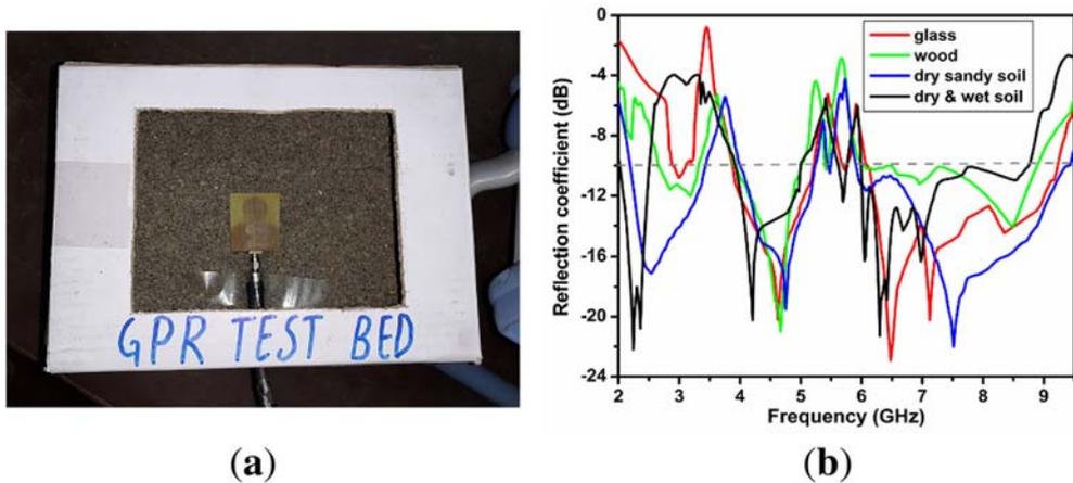
**Figure 9.** (a)  $S_{11}$  measurement set-up in proximity of soil test bed, (b) plot of reflection coefficient ( $S_{11}$ ) in proximity of various surfaces.
