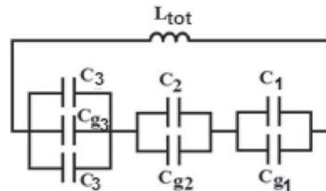
**Figure 2.** Equivalent circuit model of CSRR.
