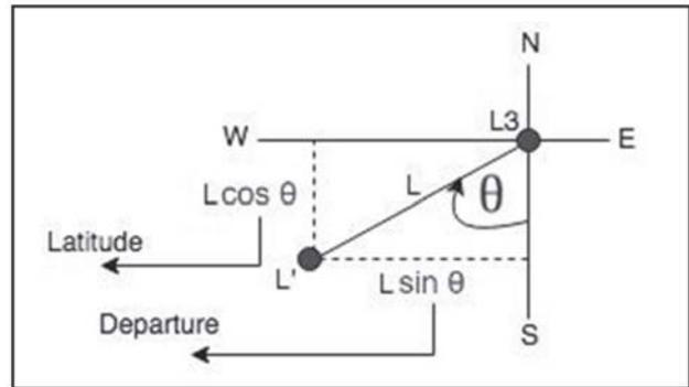
Figure 4. Illustration: Fiber-cut localization using bearing.
