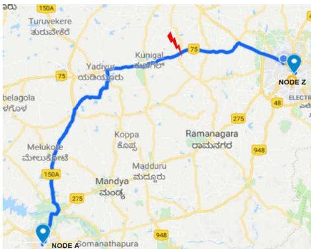
**Figure 5.** Fiber-cut localization in WEBMAP tools.
