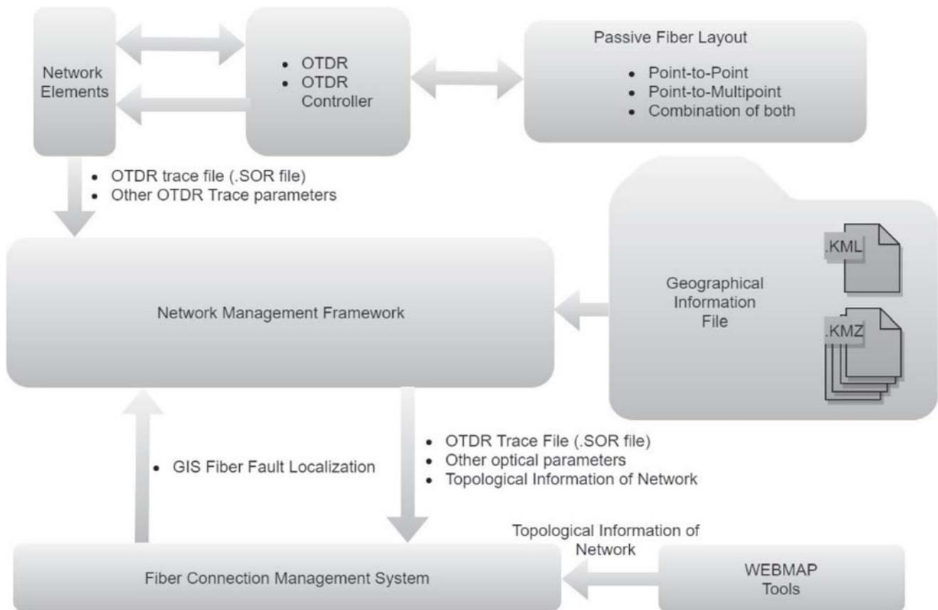
**Figure 1.** Fiber-cut localization architecture using GIS mapping.
