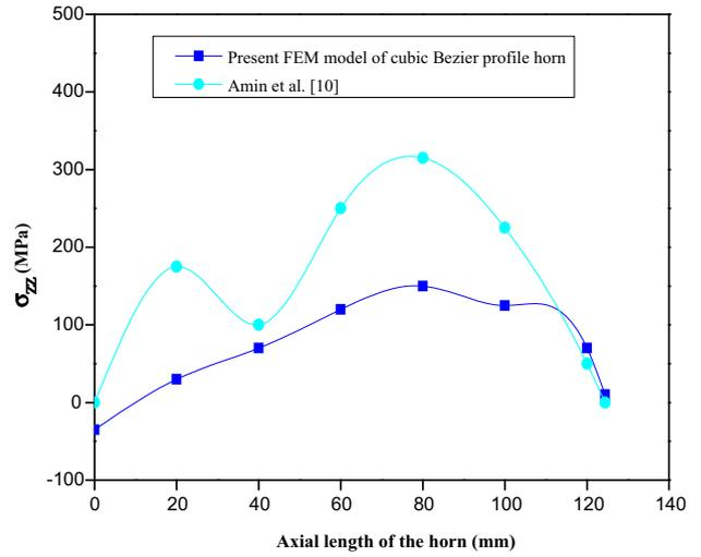
Figure 8. Axial stress ( $\sigma_{zz}$ ) variation along the axial length.
