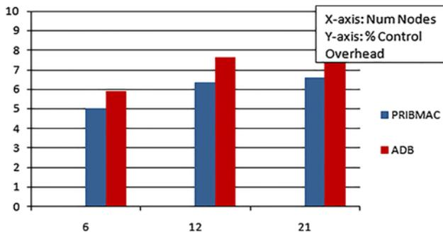
Figure 8. Control overhead of PRIB-MAC and ADB.
