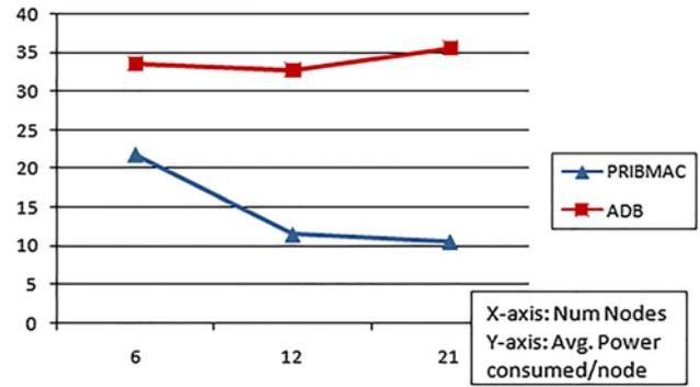
Figure 10. Average energy consumption of nodes for different network sizes in PRIB-MAC and ADB.
