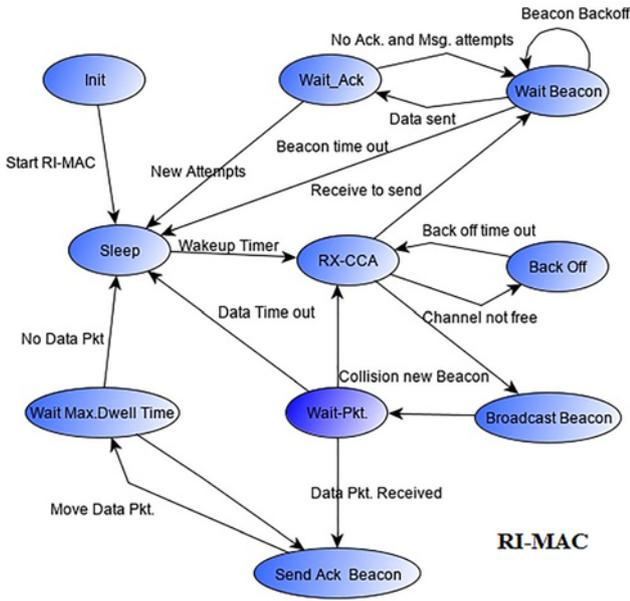
Figure 3. RI-MAC finite state machine model.
