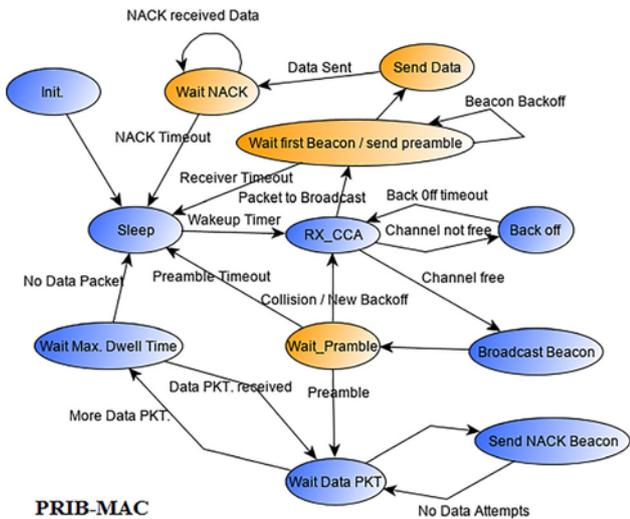
Figure 4. PRIB-MAC finite state machine model.
