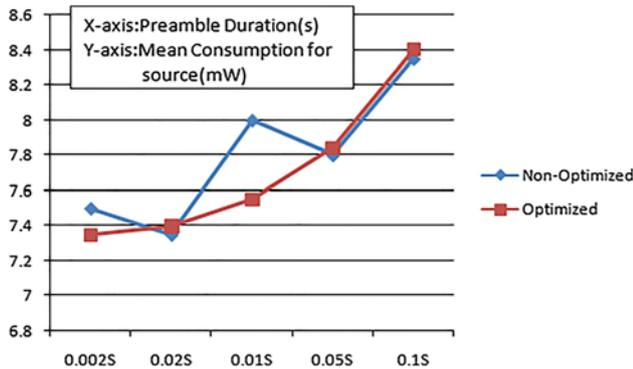
Figure 9. Mean energy consumption for different preamble durations.
