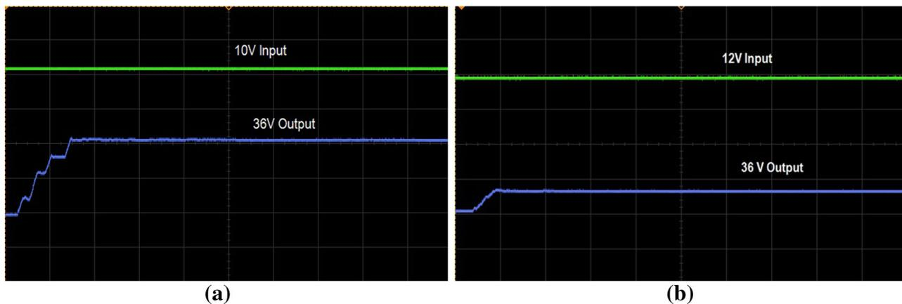
**Figure 4.** (a) Output response for 10 V input. (b) Output response for 12 V input.
