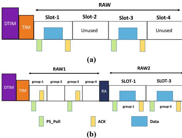
**Figure 3.** Types of RAW mechanism: (a) generic RAW mechanism and (b) triggered RAW mechanism.
