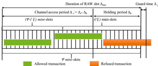
**Figure 5.** Illustration of no crossing slot case inside a RAW slot.
