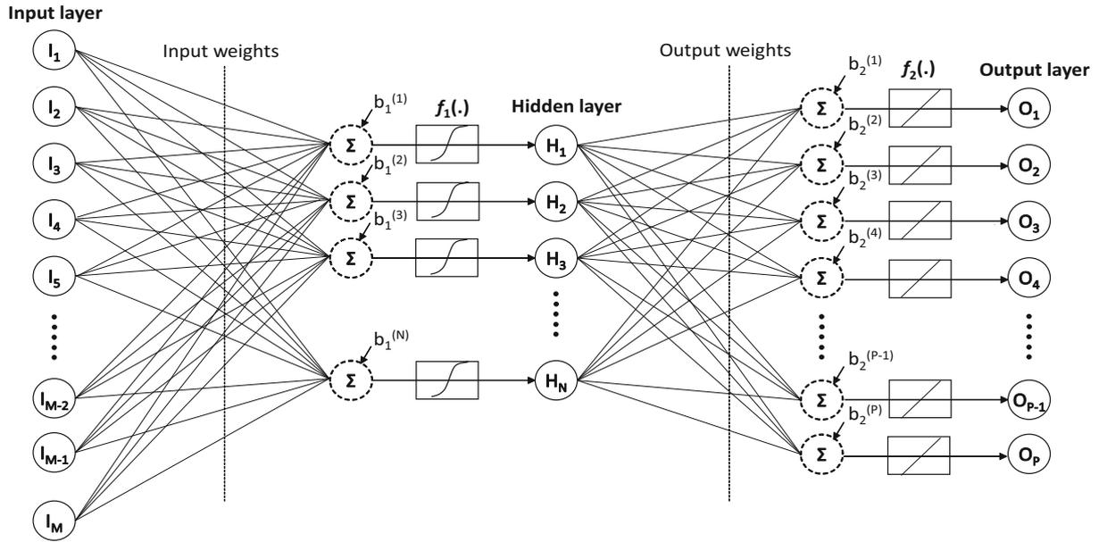
**Figure 6.** Architecture of Artificial Neural Network.
