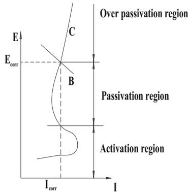
**Figure 7.** Evans diagram of passive steel corrosion in alkaline environment.
