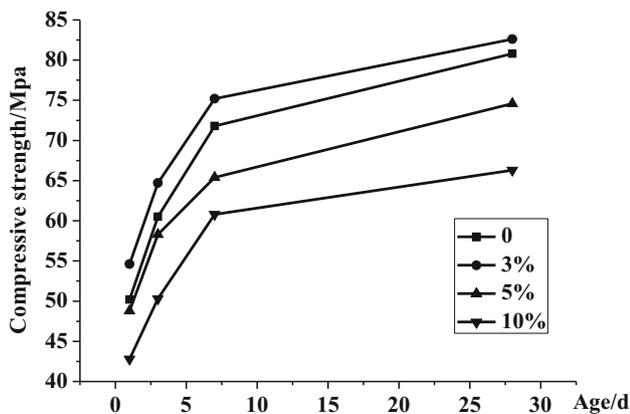
**Figure 1.** Development of compressive strength of MPC mortar.
