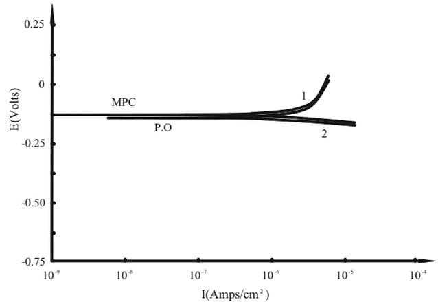
**Figure 3.** Polarization curves of reinforcing bars for 12 months.
