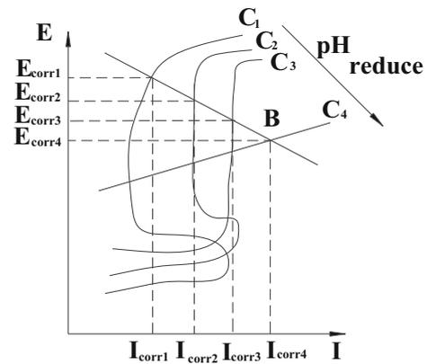
**Figure 8.** Evans diagram of effect of pH on reinforcing bar corrosion.
