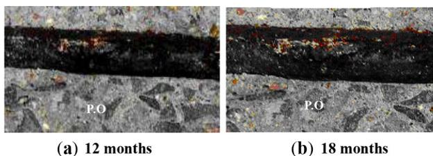
**Figure 5.** Corrosion morphology of reinforced concrete.
