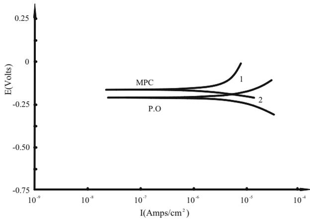
**Figure 4.** Polarization curves of reinforcing bars for 18 months.
