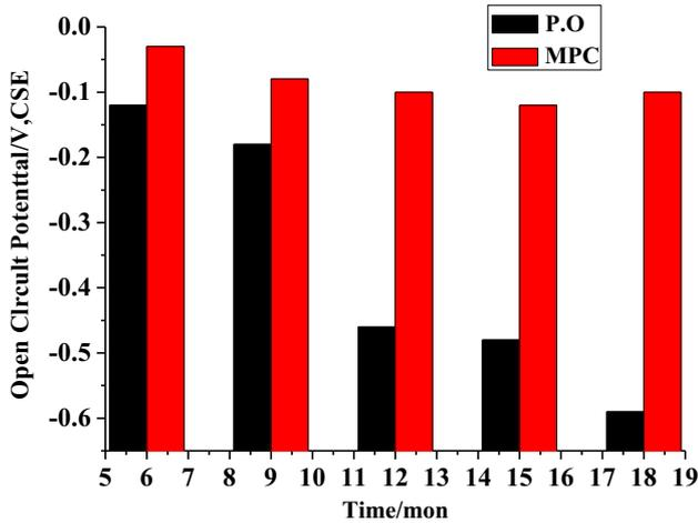
**Figure 2.** Open circuit potential changes of steel electrode system over time.
