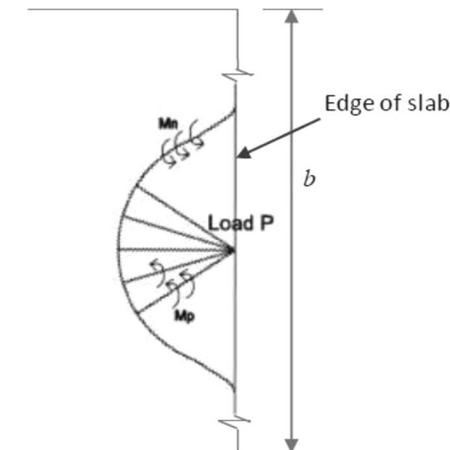
Figure 1. Cracking due to edge loads.
