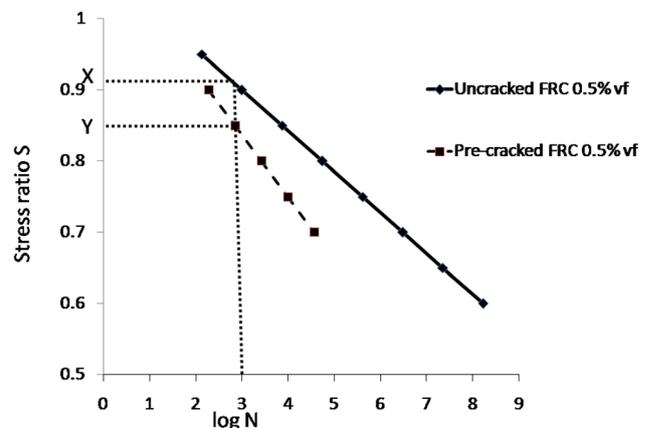
**Figure 3.** Example  $S-N$  curves for uncracked and cracked FRC.
