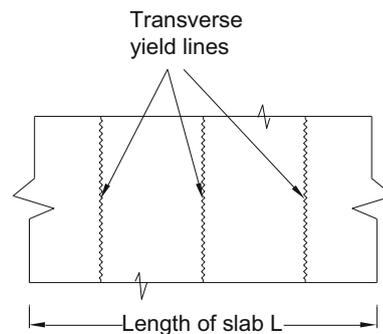
Figure 2. Cracking that occurs in narrow slabs.
