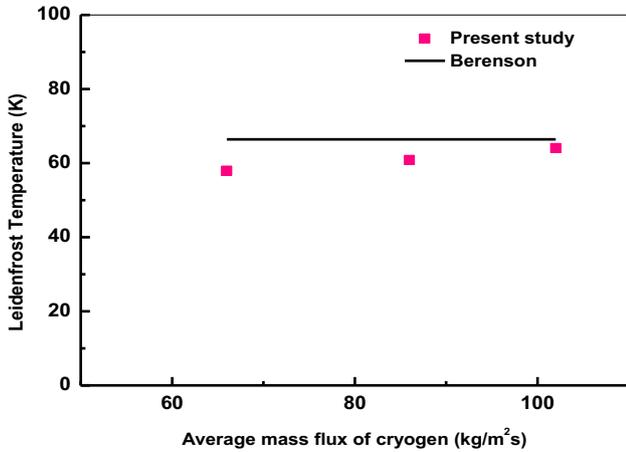
**Figure 10.** Predicted and measured Leidenfrost temperature.
