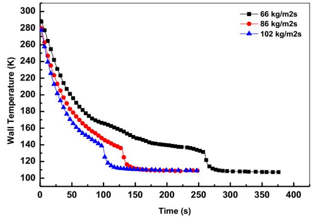
**Figure 4.** Comparison of bottom wall temperature of straight pipe at section 0.055m from inlet at 102 kg (m<sup>2</sup>.s)<sup>-1</sup>, 86 kg (m<sup>2</sup>.s)<sup>-1</sup> and 66 kg (m<sup>2</sup>.s)<sup>-1</sup>.
