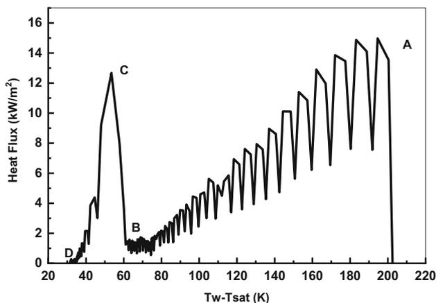
Figure 5. Variation of heat flux with wall superheat.
