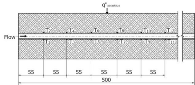
Figure 2. Thermocouple locations on test section. All units are in mm.
