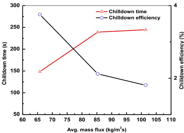
**Figure 11.** Variation of chilldown efficiency and chilldown time with mass flux.
