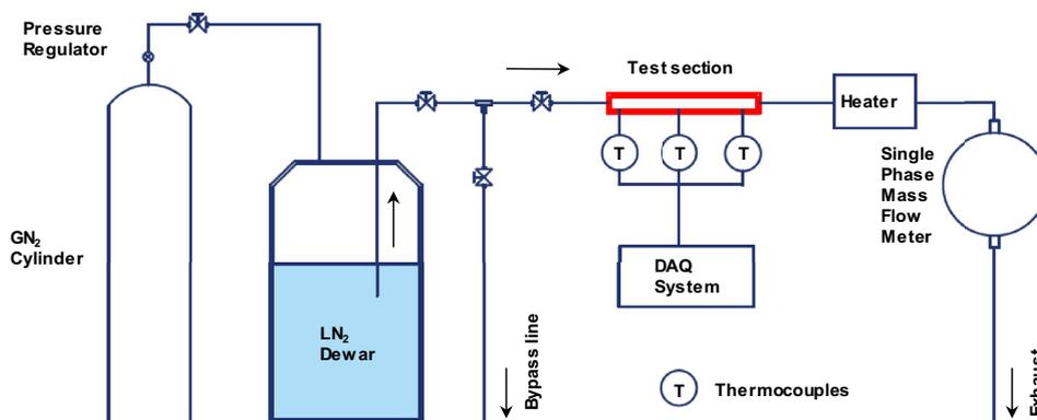
Figure 1. Layout of experimental setup for chilldown studies.
