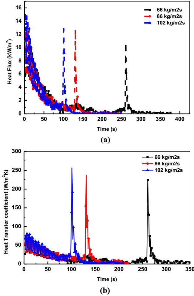
**Figure 6.** (a) Transient characteristics of heat flux, (b) inner wall heat transfer coefficient at  $z = 0.110$  m.
