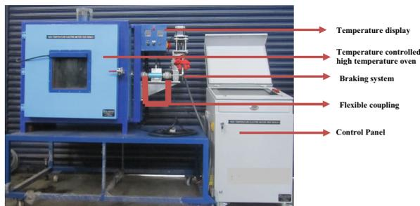
**Figure 5.** High temperature motor test bench.
