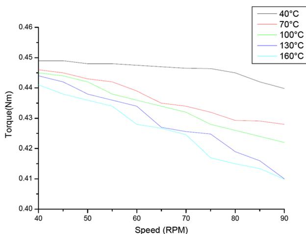
**Figure 6.** Torque–speed characteristics of stepper motor at different temperatures.
