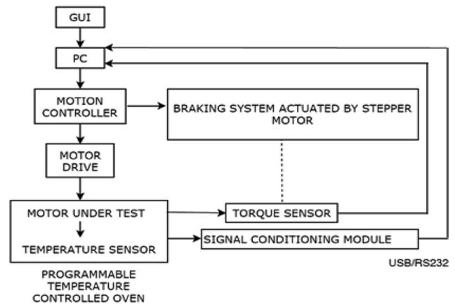
**Figure 1.** Block diagram of test bench.
