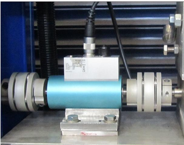
**Figure 2.** Torque sensor.
