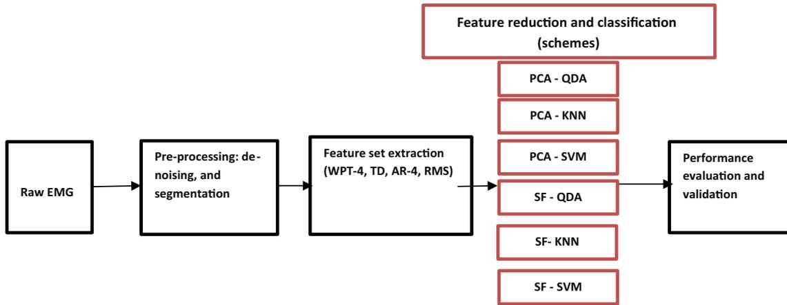
**Figure 1.** Schematic of the experimental evaluation of the proposed EMG pattern classification system.
