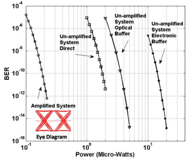
**Figure 5.** BER vs power for various switch configurations.
