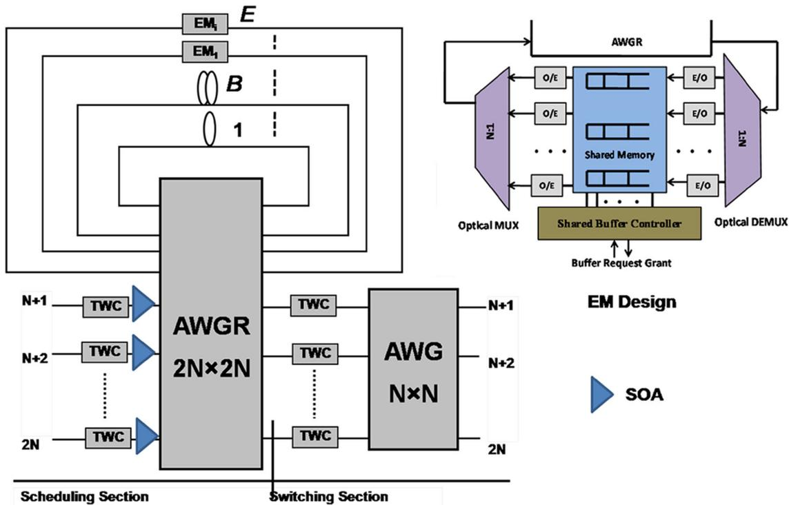
Figure 4. Design of AWG-based switch with hybrid buffer and SOAs.
