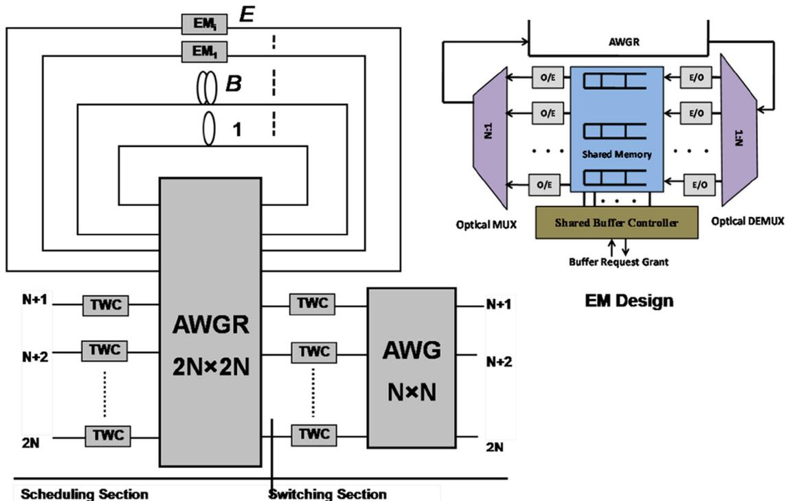
Figure 3. Design of AWG-based switch with hybrid buffer.
