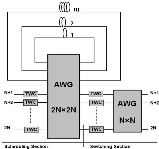
**Figure 2.** Design of AWG-based switch with optical buffer.
