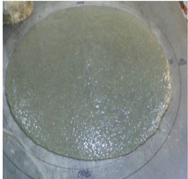
Figure 1. Slump flow spread of UHPFRC based on CARDIFRC Mix II.
