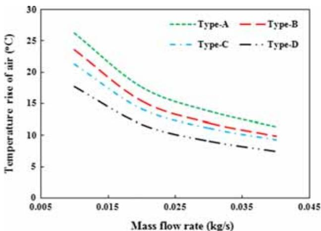
**Figure 4.** Variation of temperature rise of air with mass flow rate of air.
