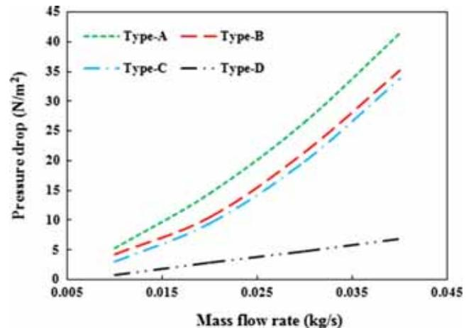
Figure 7. Variation of pressure drop with mass flow rate of air.
