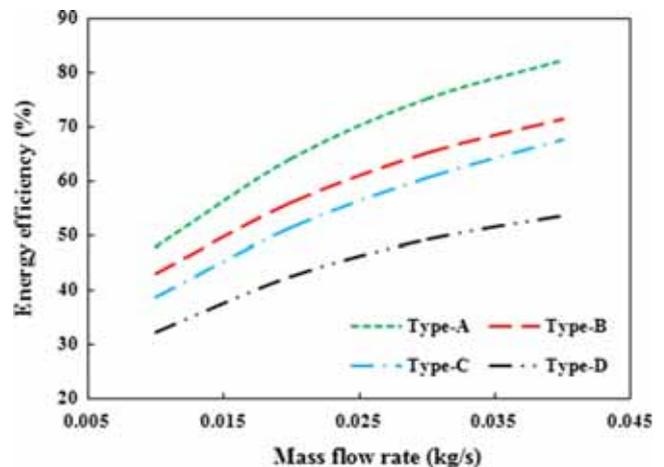
**Figure 5.** Variation of energy efficiency with mass flow rate of air.
