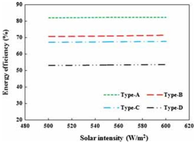
Figure 9. Variation of energy efficiency with solar intensity.
