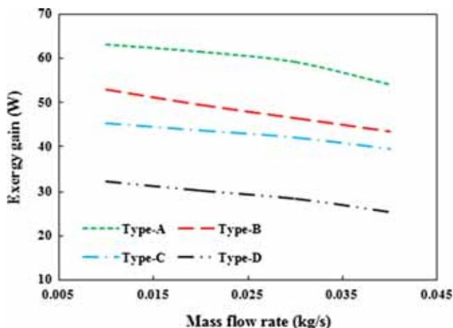
Figure 6. Variation of exergy gain with mass flow rate of air.
