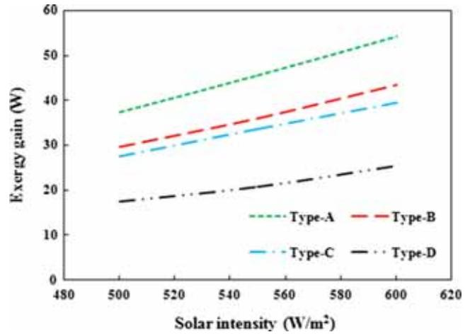
Figure 10. Variation of exergy gain with solar intensity.
