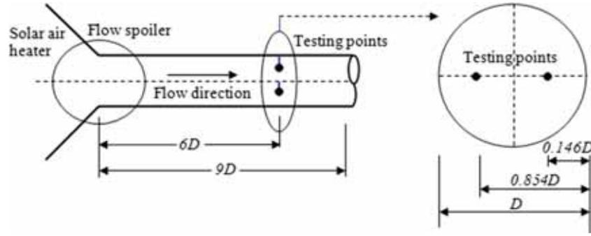
**Figure 3.** Air velocity measurement locations and testing points.
