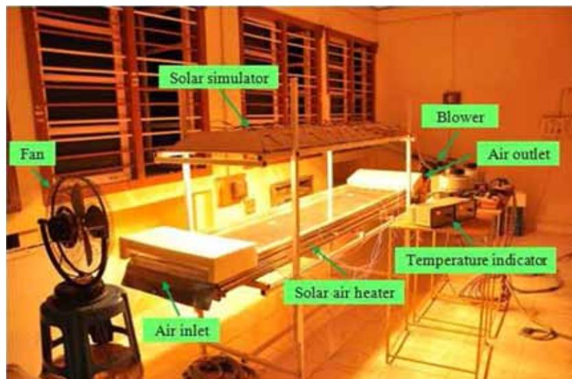
Figure 1. Photographic view of experimental setup.
