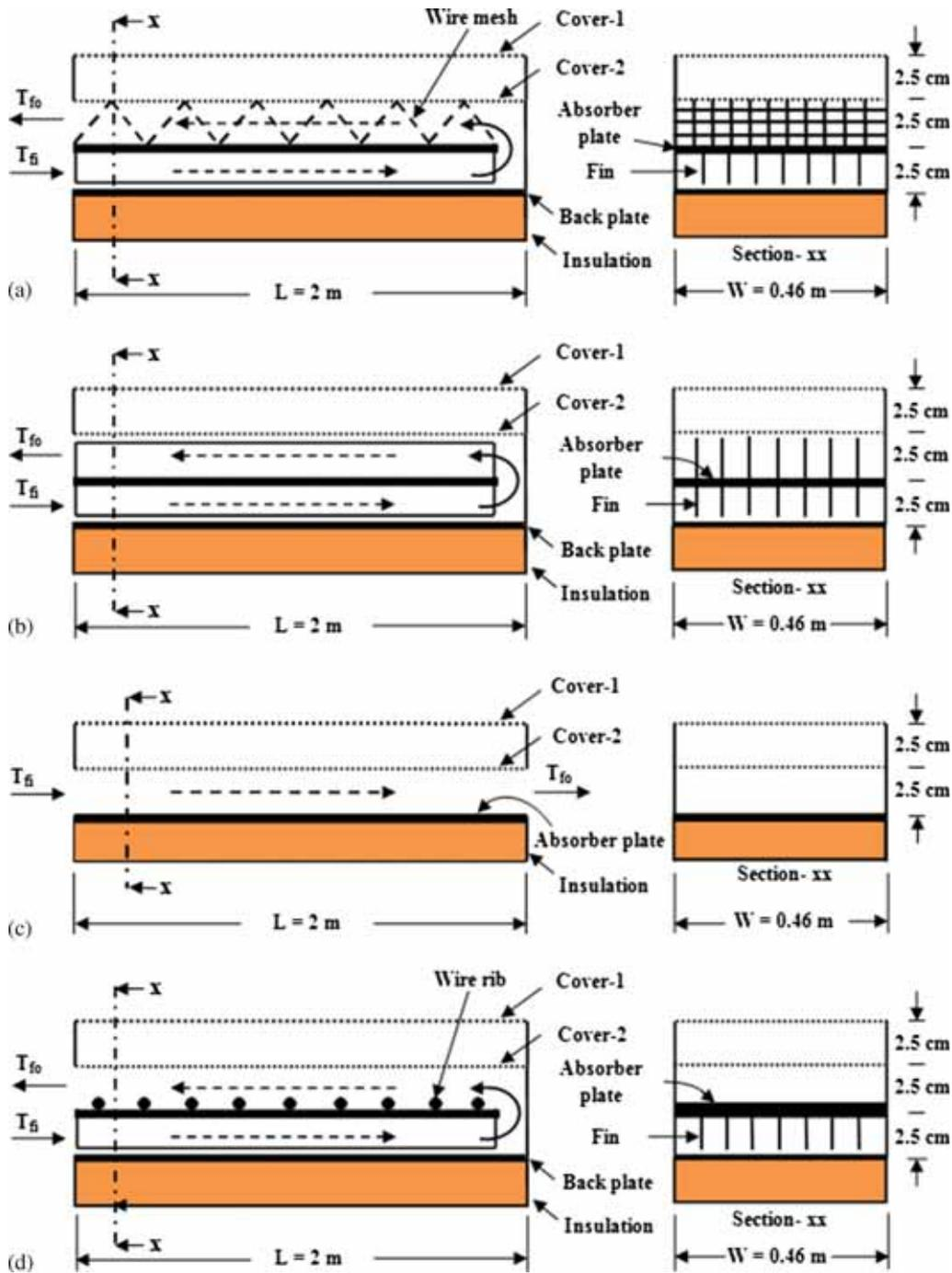
**Figure 2.** Various configuration of solar air heaters: (a) V-corrugated wire mesh double pass solar air heater with longitudinal fins (type-A), (b) Finned plate double pass solar air heater with longitudinal fins (type-B), (c) Roughened plate double pass solar air heater with longitudinal fins (type-C), (d) Conventional flat plate single pass solar air heater (type-D).
