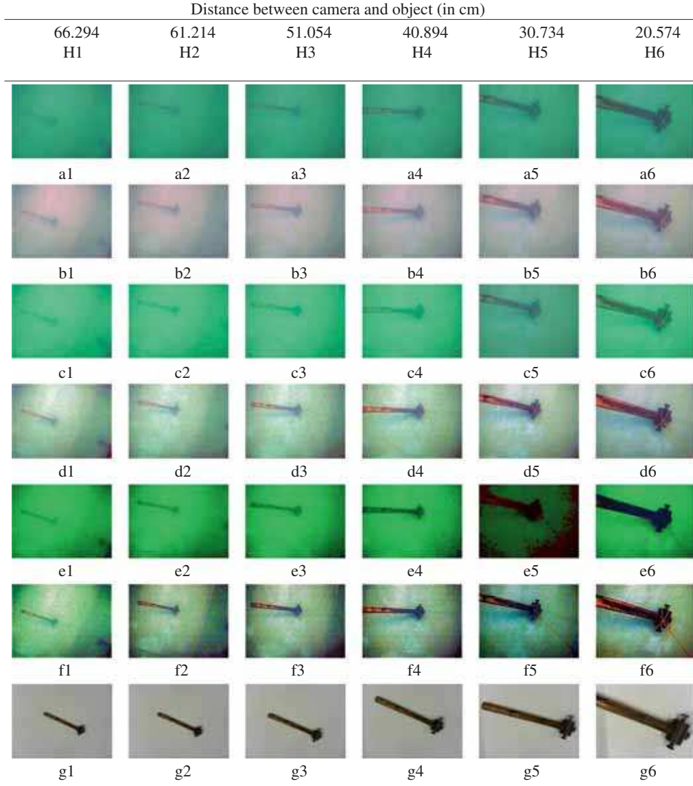
Figure 7. Hammer image: H1–H6: Original images of Hammer according with distances, specified at the top. (a1–a6) Original images; enhanced Images using – (b1–b6) GW; (c1–c6) WP; (d1–d6) APE; (e1–e6) UCM; (f1–f6) RYPro; (g1–g6) out-of-water (in air) images.
