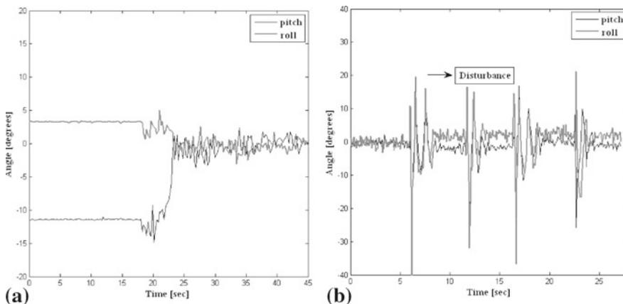
**Figure 9.** (a) System response to an initial condition. (b) System response to random disturbances.
