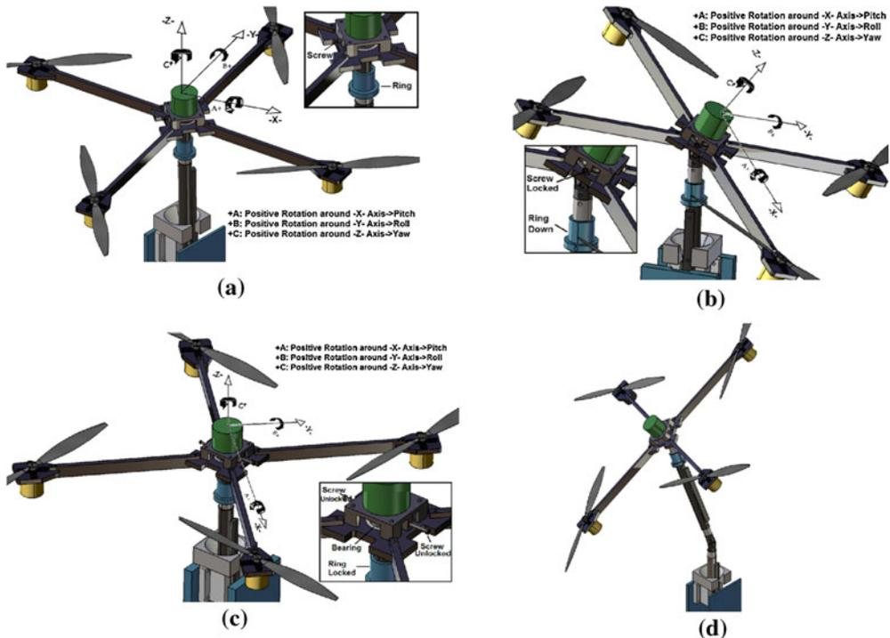
**Figure 2.** (a) Vertical elevation control while locking rings for pitch/yaw/roll motion in place. (b) Pitch/Roll control while locking screw for yaw motion in place. (c) Yaw control while locking rings for pitch/roll motion in place. (d) Spatial motion of the quadrotor in the stationary testbed.
