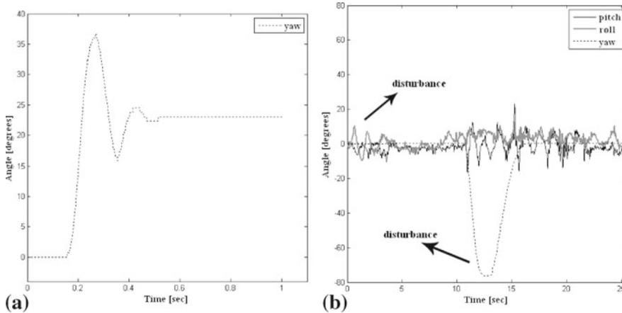
**Figure 10.** (a) Yaw response to a step command of 23 degrees. (b) Pitch, roll and yaw's control under random disturbances.
