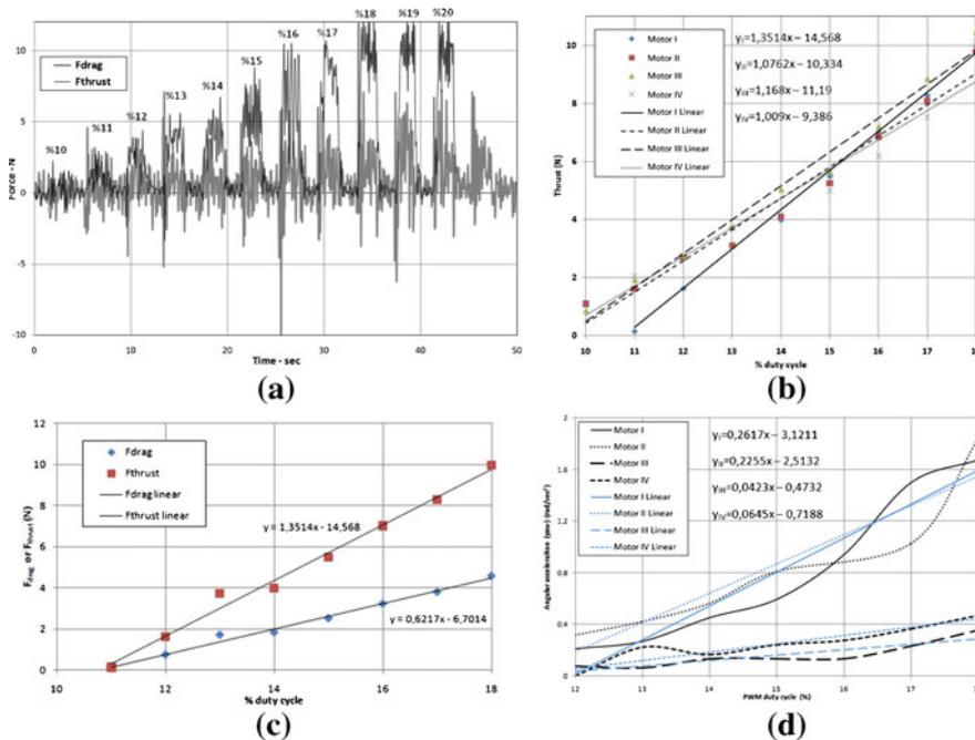
**Figure 5.** (a) Drag and thrust force outputs of motor I for several PWM % duty cycles. (b) Static thrust of the motors for increasing PWM % duty cycle for selecting motor pairs. (c) Motor I thrust and drag relationship. (d) Max yaw accelerations based on motor input PWM percent duty cycles.
