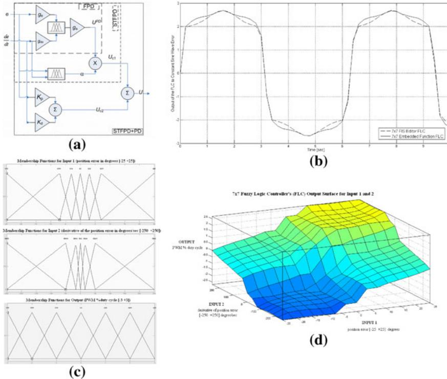
**Figure 8.** (a) Block diagram of the control algorithms. (b) Output of the  $7 \times 7$  FIS Editor FLC and of the  $7 \times 7$  embedded function FLC. (c) FLC Membership Functions. (d)  $7 \times 7$  Fuzzy logic controller's (FLC) output surface for input 1 and 2.
