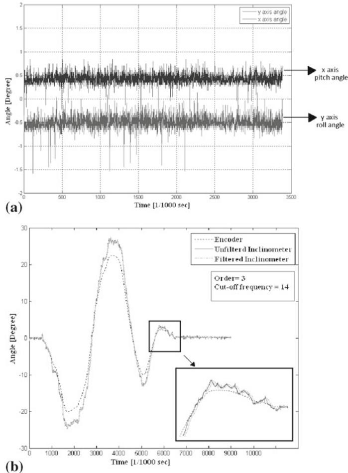
**Figure 6.** (a) Noise observed at the output of the inclinometer when it is parallel to the ground. (b) Filtered and unfiltered inclinometer's comparison.
