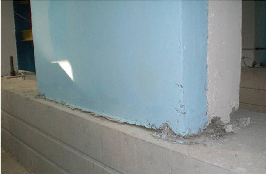
**Figure 10.** Concordant behaviour of the connecting column and the new shear wall.
