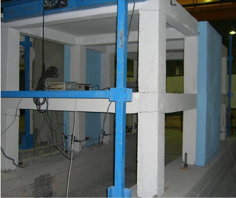
Figure 11. Damaged SM after the test.
