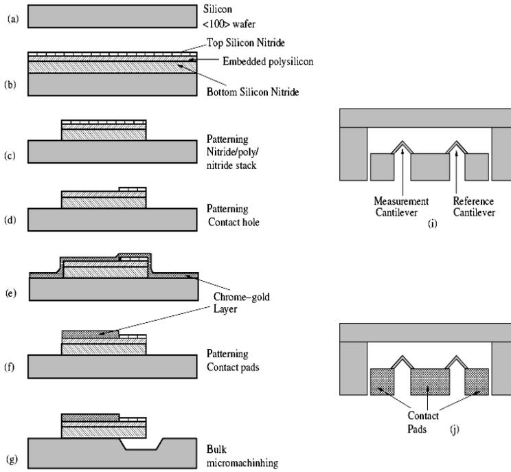
**Figure 3.** Process flow highlighting the main steps in fabricating the piezo-resistive cantilevers.
