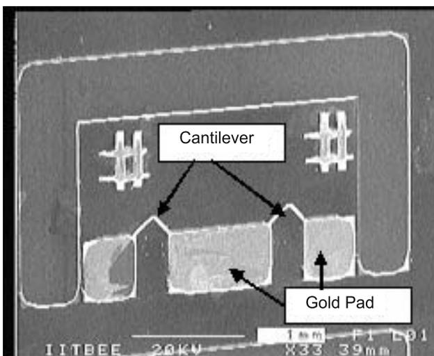
**Figure 5.** Full die showing the piezo-resistive cantilevers connected in half Wheatstone bridge configuration.
