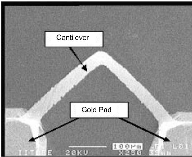
**Figure 4.** A released nitride/polysilicon/nitride cantilever.
