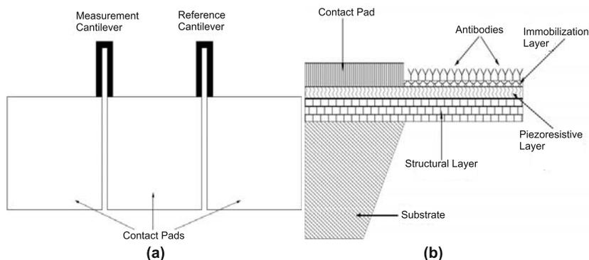
**Figure 1.** Schematic of the piezo-resistive cantilever (a) plan view, (b) cross-sectional view.
