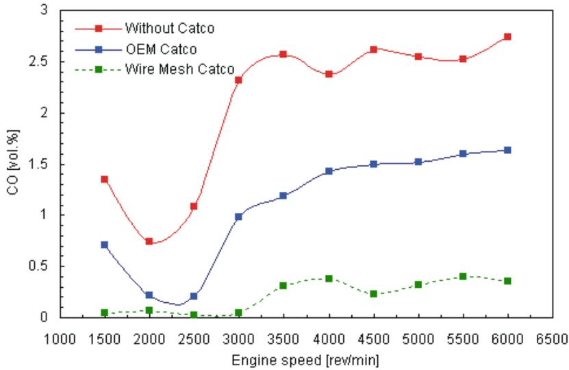
**Figure 9.** CO emission versus engine speed (with and without catalytic converter) at WOT.
