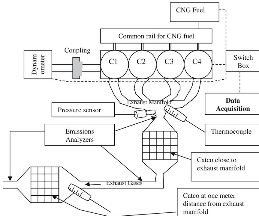
**Figure 7.** Schematic diagram of catco(s) on the engine exhaust pipe.
