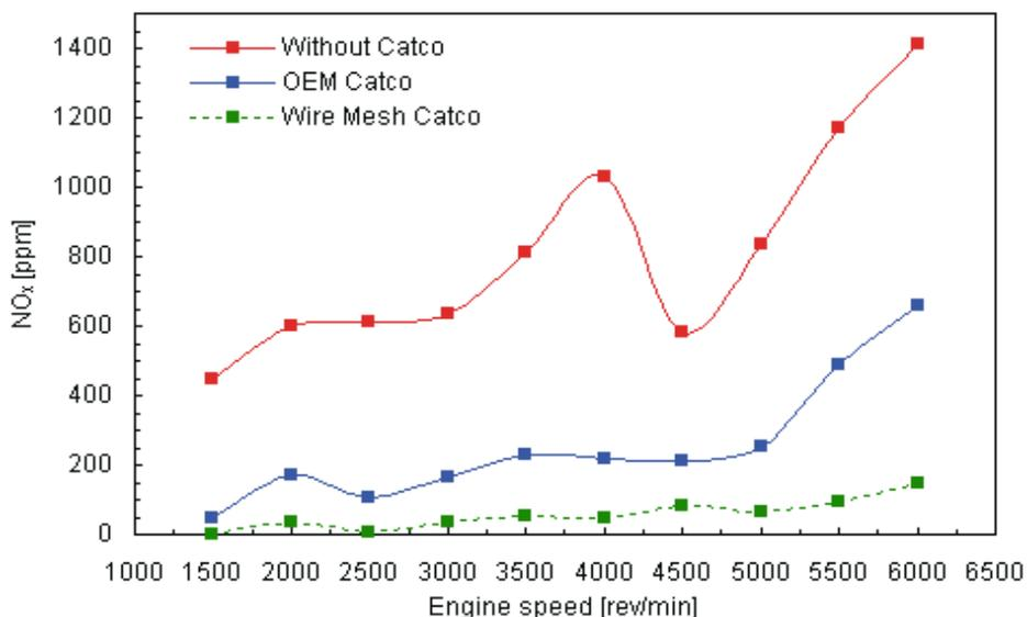
**Figure 8.**  $\text{NO}_x$  emission versus engine speed (with and without catalytic converter) at WOT.
