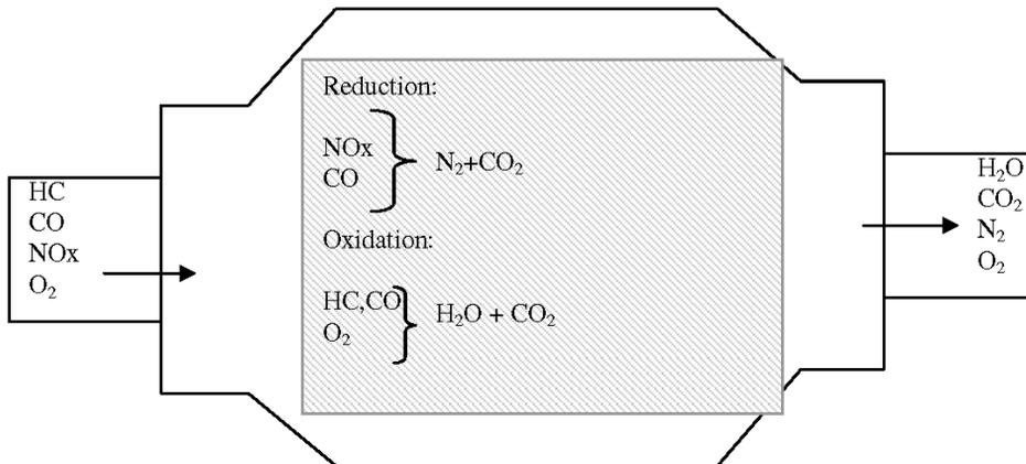
**Figure 6.** Oxidation and reduction process into catalytic converter.
