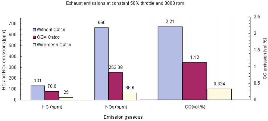
Figure 11. HC, CO and NO<sub>x</sub> emissions at constant 50% throttle and 3000 rpm.
