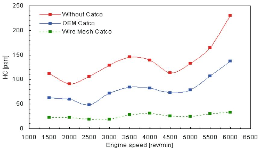
**Figure 10.** HC emission versus engine speed (with and without catalytic converter) at WOT.
