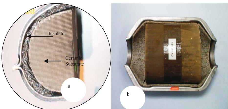
**Figure 3.** (a) Original proton honeycomb ceramic substrate and (b) casing for honeycomb ceramic substrate.
