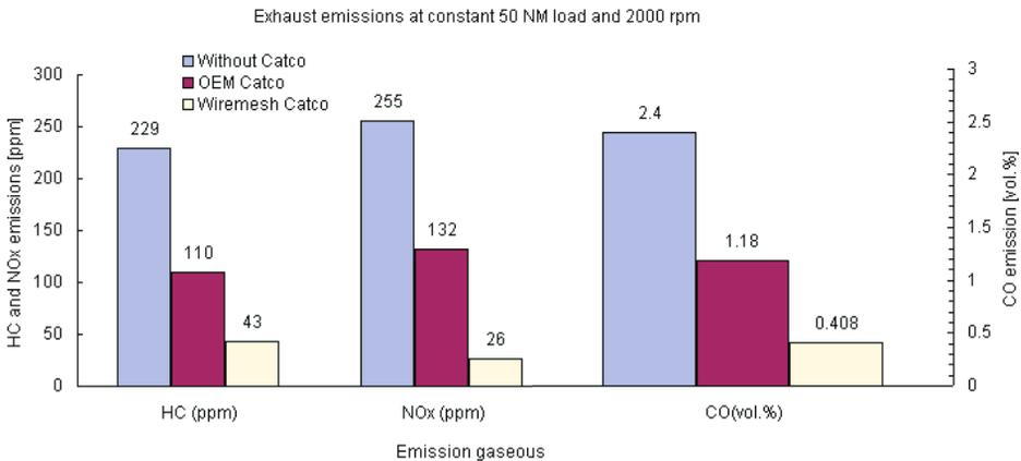
Figure 12. HC, CO and NO<sub>x</sub> emissions at constant 50 Nm load and 2000 rpm.
