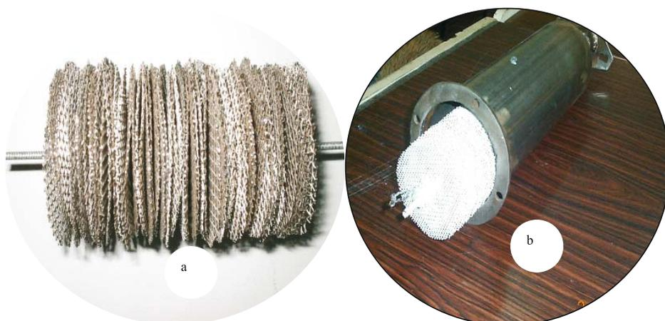
**Figure 2.** (a) Wire mesh substrate configurations, (b) wire mesh substrate in catalytic converter casing.
