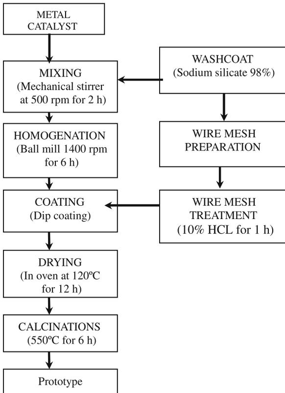
**Figure 5.** Summary of catalyst and substrate preparation.
