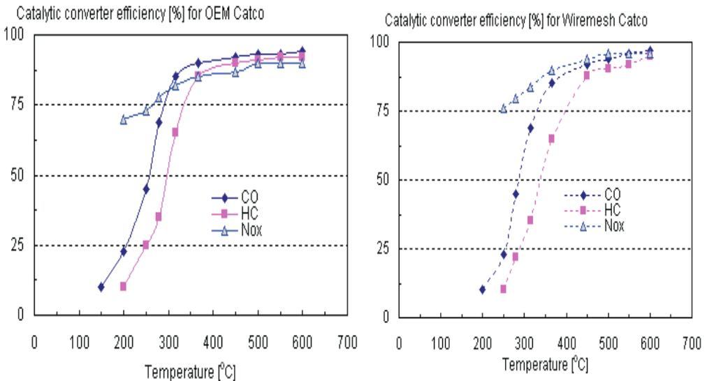
**Figure A1.** Catalytic converter efficiency versus temperature at 50% throttle condition.
