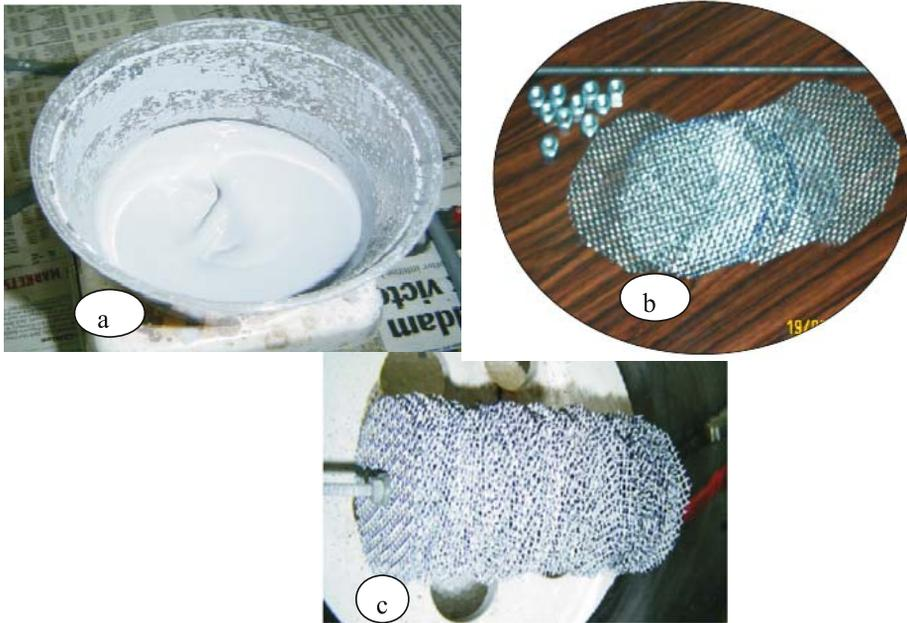
**Figure 1.** (a) Finished mixture of metal catalyst and wash coat slurry, (b) wire mesh substrates are cut in circular shape, (c) arranged calcined wire mesh substrate.
