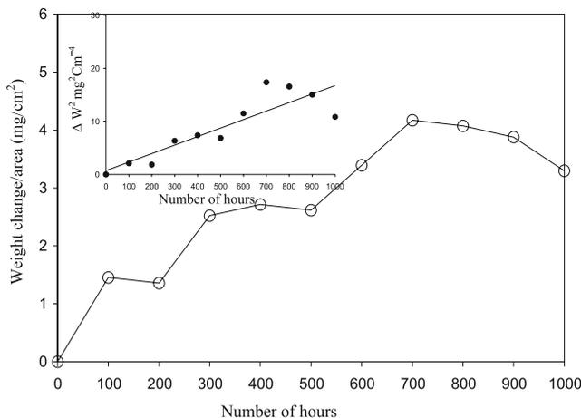
**Figure 1.** Weight change vs. time plots for Superni-75 during cyclic study in the real service environment of the coal-fired boiler. Insert is fitted for  $(\text{weight change}/\text{area})^2$  vs time plots.
