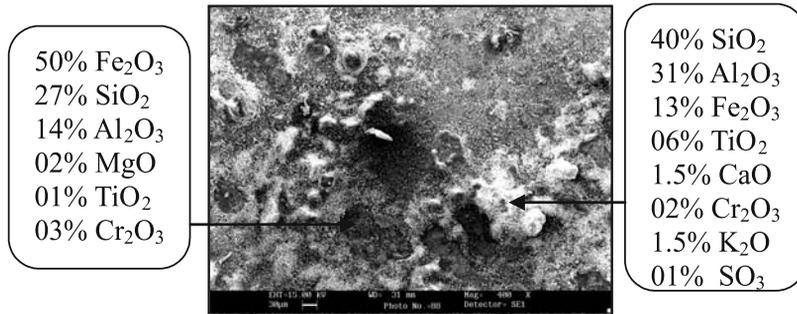
**Figure 4.** SEM/EDAX analysis showing elemental composition (wt.%) for the Superni-75 after 1000 h exposure to platen superheater zone of the coal-fired boiler at 900°C.
