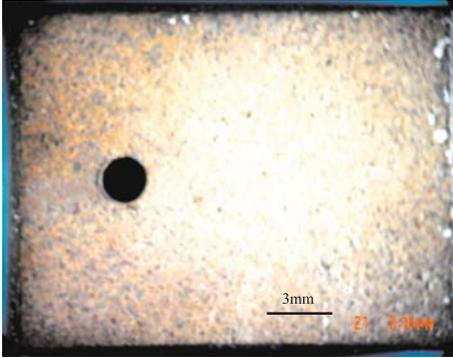
**Figure 2.** Macrographs of the Superni-75 after 1000 h exposure to platen superheater zone of the coal-fired boiler at 900°C.
