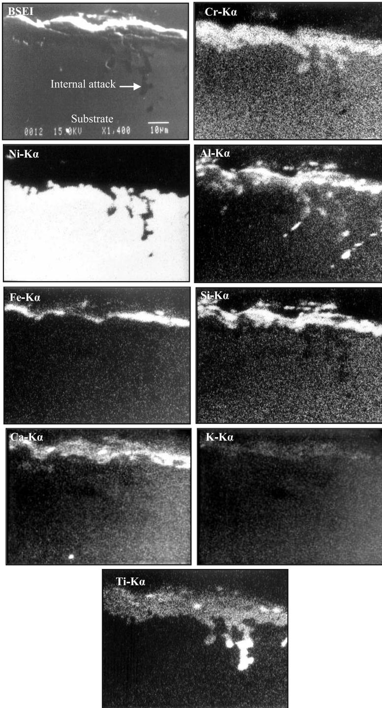
**Figure 6.** Composition image (BSEI) and X-ray mappings across the cross-section of Superni-75 after 1000 h exposure to platen superheater zone of the coal-fired boiler at 900°C.
