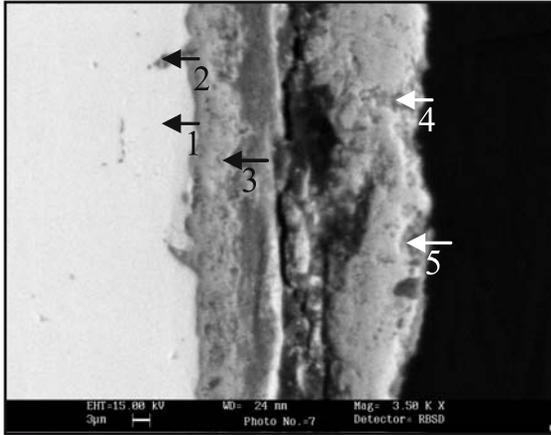
**Figure 5.** Oxide scale morphology and variations of elemental composition (wt%) across the cross section of Superni-75 after 1000 h exposure to platen superheater zone of the coal-fired boiler at 900°C.
