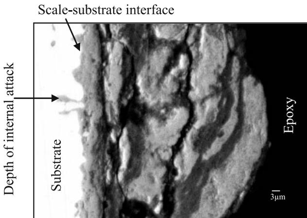
**Figure 3.** BSE image for the Superni-75 after 1000 h exposure to platen superheater zone of the coal-fired boiler at 900°C.
