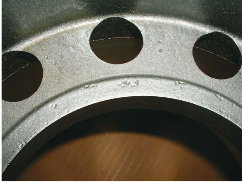
Figure 1. Blow-holes in cast component.
