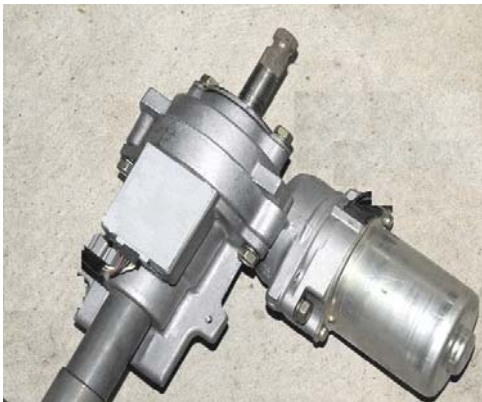
Figure 7. Gear box with motor.
