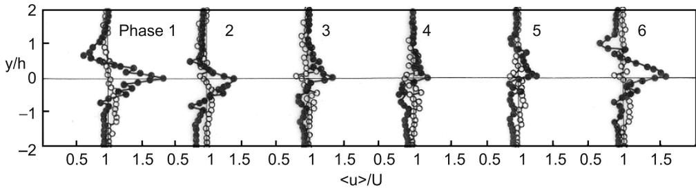
**Figure 9.** Ensemble-average velocity profiles for  $C_q = 0.075$  and  $F = 1.82$  ( $\circ$  :  $x/h = 2$ ,  $\bullet$  :  $x/h = 5$ ).
