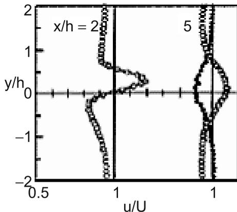
**Figure 7.** Mean velocity profiles with steady blowing  $C_q = 0.129$  ( $\circ$ ) and  $C_q = 0$  ( $\bullet$ ) from Sharma & Sahoo (1998).
