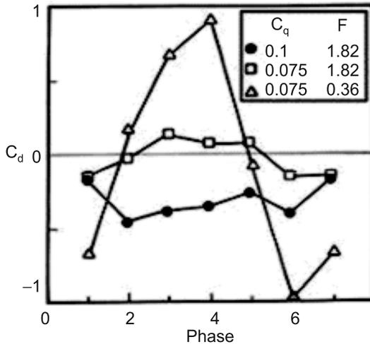
**Figure 12.** Phasewise variation of drag coefficient.
