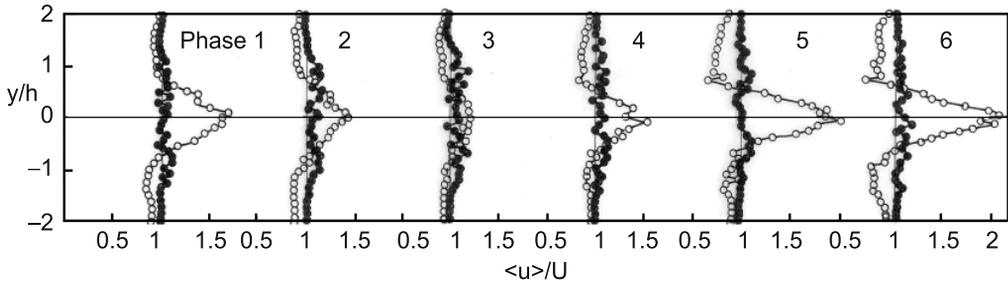
**Figure 10.** Ensemble-average velocity profiles for  $C_q = 0.1$  and  $F = 1.82$  ( $\circ$  :  $x/h = 2$ ,  $\bullet$  :  $x/h = 5$ ).
