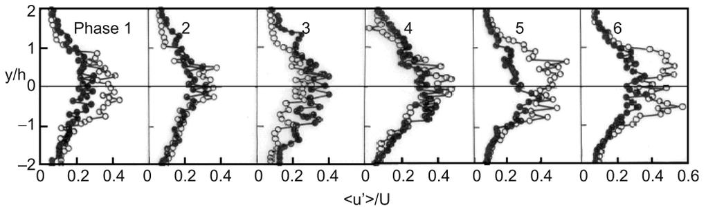
**Figure 11.** Phasewise turbulence profiles for  $C_q = 0.1$  and  $F = 1.82$  ( $\circ$  :  $x/h = 2$ ,  $\bullet$  :  $x/h = 5$ ).
