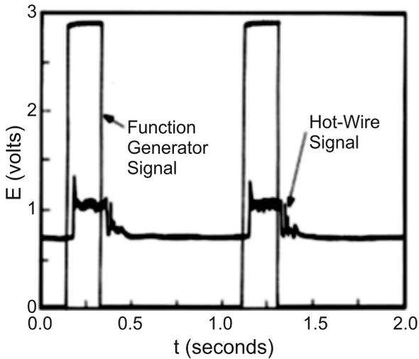
**Figure 2.** Signals from the function generator and hot-wire exhibit responsiveness of solenoid valve.
