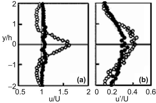
**Figure 6.** Wake profiles: (a) mean velocity and (b) turbulence with  $C_q = 0.1$  forced at  $F = 1.8$  ( $\circ$  :  $x/h = 2$ ,  $\bullet$  :  $x/h = 5$ ).
