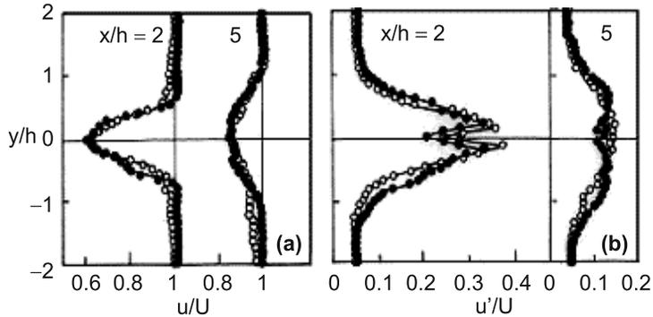
**Figure 4.** Unforced wake profiles: (a) mean velocity and (b) turbulence. ( $\circ$  :  $U = 4.1$  m/s,  $\bullet$  :  $U = 1.1$  m/s).
