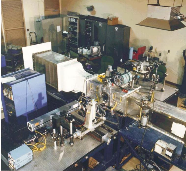
**Figure 1.** A view of the compressible dynamic stall facility.
