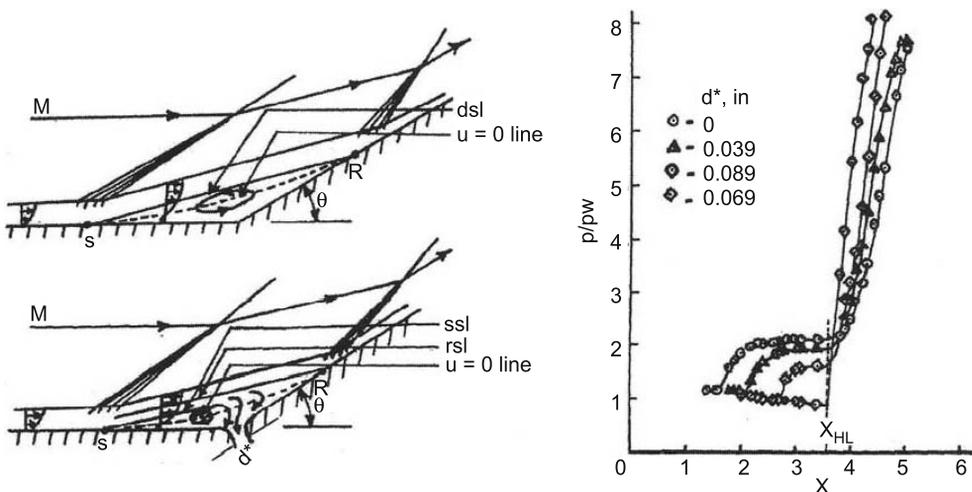
**Figure 2.** Flow separation at a compression corner and streamwise pressure distributions with suction (from Ball & Korkegi 1968).
