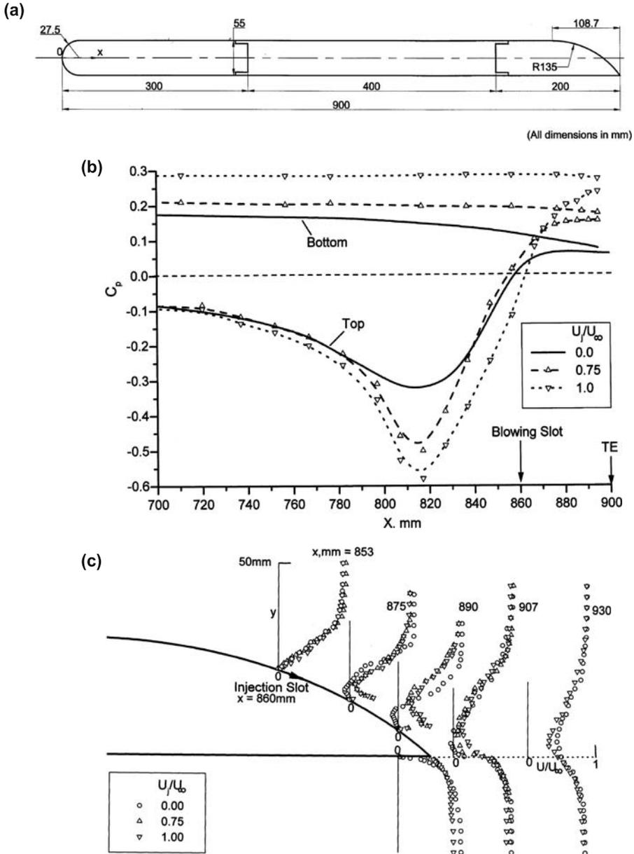
**Figure 4.** Control of trailing-edge separated flow by tangential blowing inside bubble. (a) Geometric details of flat plate-contoured aft-section model. (b) Effect of blowing on model static pressure distributions. (c) Effect of blowing on mean velocity profiles in the separated zone.
