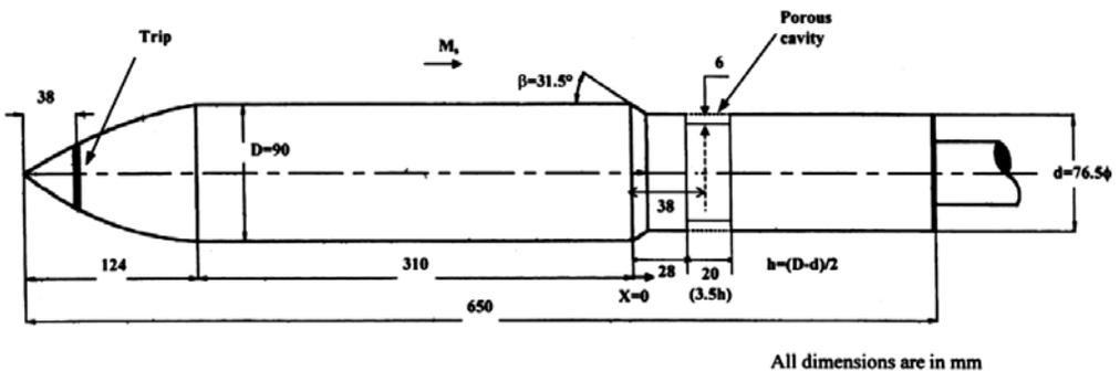
**Figure 6.** Geometric details of a generic axisymmetric body.
