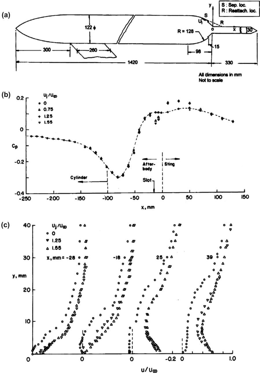
**Figure 3.** Separation control by tangential blowing inside bubble. (a) Axisymmetric model. (b) Effect of blowing on surface distributions. (c) Effect of blowing on mean velocity profiles in separated region.
