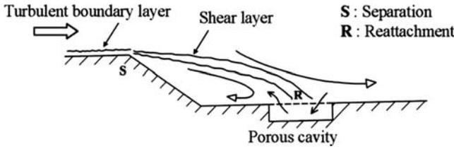
**Figure 5.** Schematic of passive control concept for reattaching flow.
