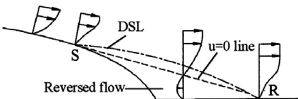
**Figure 1.** Schematic of main features of a 2D turbulent separated flow.
